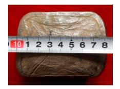
**Figure 6.** External appearance of Ti-43Al-2Cr-1.5Mn-0.2Y alloy fabricated by MDF with a reduction of 30% per pass.
