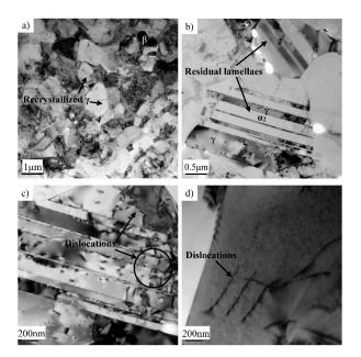
**Figure 8.** Transmission electron microscope (TEM) images showing the microstructures of Ti-43Al-2Cr-1.5Mn-0.2Y alloy after third pass forging. (a) DRX region, (b) residual lamellae, and (c,d) high-density dislocation in the  $\gamma$  phase
