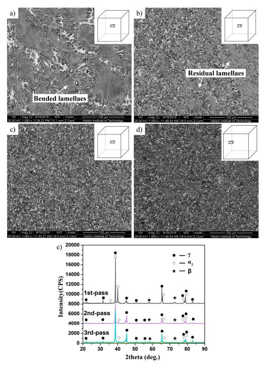
**Figure 5.** Effect of forging pass (30% reduction per pass) on microstructures of Ti-43Al-2Cr-1.5Mn-0.2Y alloy. (**a**) One pass/center area, (**b**) two passes/center area, (**c**) three passes/center area, and (**d**) three passes/bulging area. (**e**) X-ray diffraction (XRD) patterns after different forging cycles.
