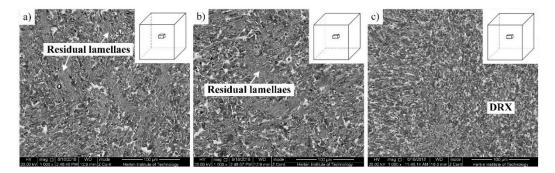
**Figure 4.** Effect of forging temperature on microstructures of Ti-43Al-2Cr-1.5Mn-0.2Y alloy. (**a**) 1150 °C, (**b**) 1200 °C, (**c**) 1250 °C.
