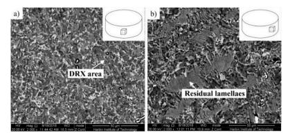
**Figure 3.** Microstructures of Ti-43Al-2Cr-1.5Mn-0.2Y alloy fabricated by SDF with a reduction of 60%. (a) Center area, (b) Bulging area.
