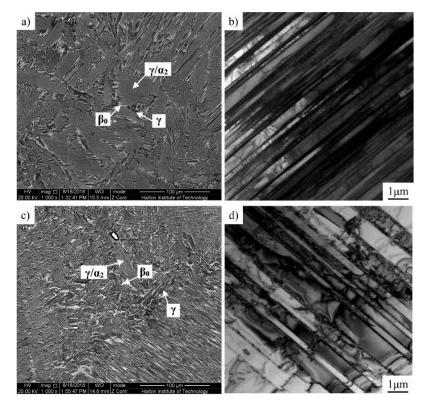
**Figure 2.** Microstructures of the as-cast Ti-43Al-2Cr-1.5Mn-0.2Y alloy. (**a**,**b**) initial condition, and (**c**,**d**) after homogenization treatment.
