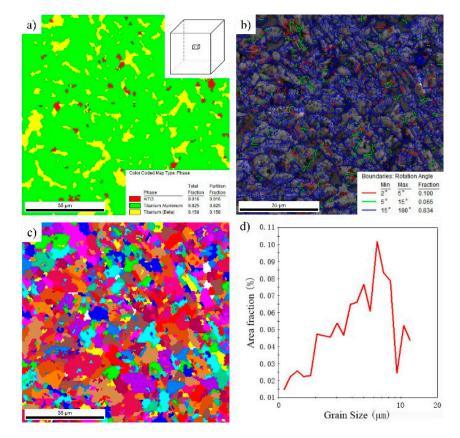
**Figure 7.** Electron back-scattered diffraction (EBSD) maps showing the microstructure of Ti-43Al-2Cr-1.5Mn-0.2Y alloy produced in three-steps forging. (a) Phase composition, (b) grain boundary characteristic, (c) grain map, and (d) grain size distribution.
