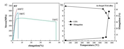
**Figure 9.** Tensile properties of the multi-directional forged TiAl alloy. (a) Tensile curves, and (b) variation of ultimate tensile strength (UTS) and  $\delta$  with temperature.
