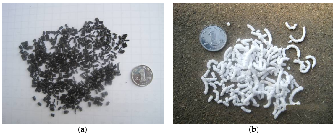
Figure 1. Additives: (a) Granular Polymer Durable additive (GPDa); (b) Styrene-Butadiene-Styrene (SBS).
