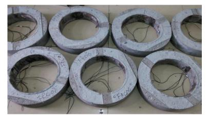
Figure 5. Specimens for the plat-ring-type test.
