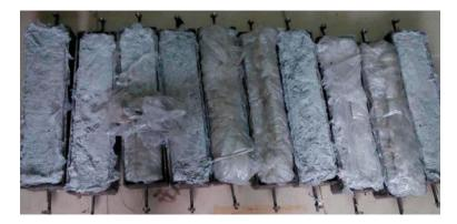
Figure 7. Specimens for the free shrinkage test.
