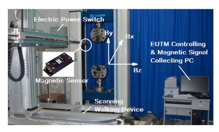
**Figure 1.** Electric universal testing machine (EUTM) and automatic triaxial self-magnetic flux leakage (SMFL) signal acquisition device.
