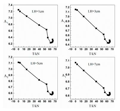
Figure 7. A<sub>T</sub>-T diagram of the By signal of 12 mm diameter TSB.
