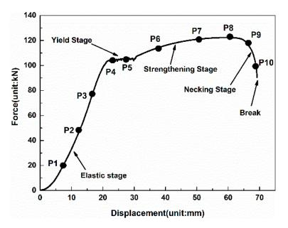
Figure 2. Targeted loading displacement (TLD) points selection indication from the tensile-displacement curve.
