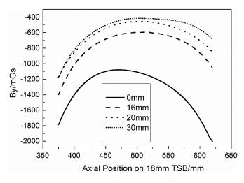
Figure 6. Axial scanning test results of some TLDs of 18 mm TSB at LH = 3 cm.
