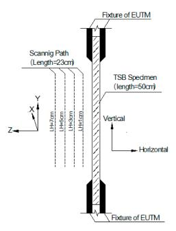
Figure 3. Scanning path diagram of magnetic sensor in the axial scanning test.
