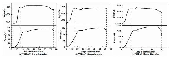
**Figure 4.** Variation of By signal with displacement during the loading of 1# TSB. (**a**) TSB of 12 mm diameter, (**b**) TSB of 16 mm diameter and (**c**) TSB of 18 mm diameter.
