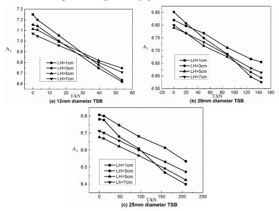
**Figure 8.** The linear section of A<sub>T</sub>-T graphs under different LHs for different TSB diameters. (**a**) 12 mm diameter TSB; (**b**) 20 mm diameter TSB; (**c**) 25 mm diameter TSB.
