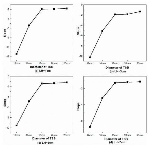
**Figure 12.** The slope of the linear segment in the  $A_T$ -T diagram with different TSB diameters in the axial scanning test. (a) LH = 1 cm, (b) LH = 3 cm, (c) LH = 5 cm and (d) LH = 7 cm.
