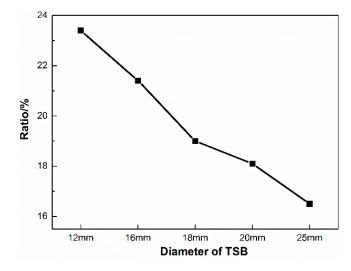
**Figure 10.** The ratio of the tensile force corresponding to the peak value on the first derivative curve of the By signal to the yield tension with different TSB diameters of the elastic stage in the fixed-point monitoring test (%).
