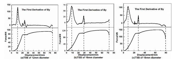
**Figure 5.** The variation of the first derivative of the By signal with the loading displacement. (**a**) TSB of 12 mm diameter, (**b**) TSB of 16 mm diameter and (**c**) TSB of 18 mm diameter.
