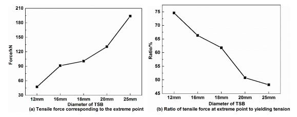
**Figure 9.** The tensile force corresponding to the extreme point on the By curve in the fixed-point monitoring test with different TSB diameters. (a) Tensile force corresponding to the extreme point, (b) Ratio of tensile force at extreme point to yielding tension.
