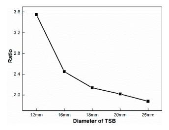
**Figure 11.** The ratio of the two peak values on the first derivative curve of the By signal in the fixed-point monitoring test with different TSB diameters.
