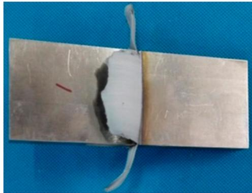
Figure 4. Morphology of the  $Ti_3Al$  joint after LFW.
