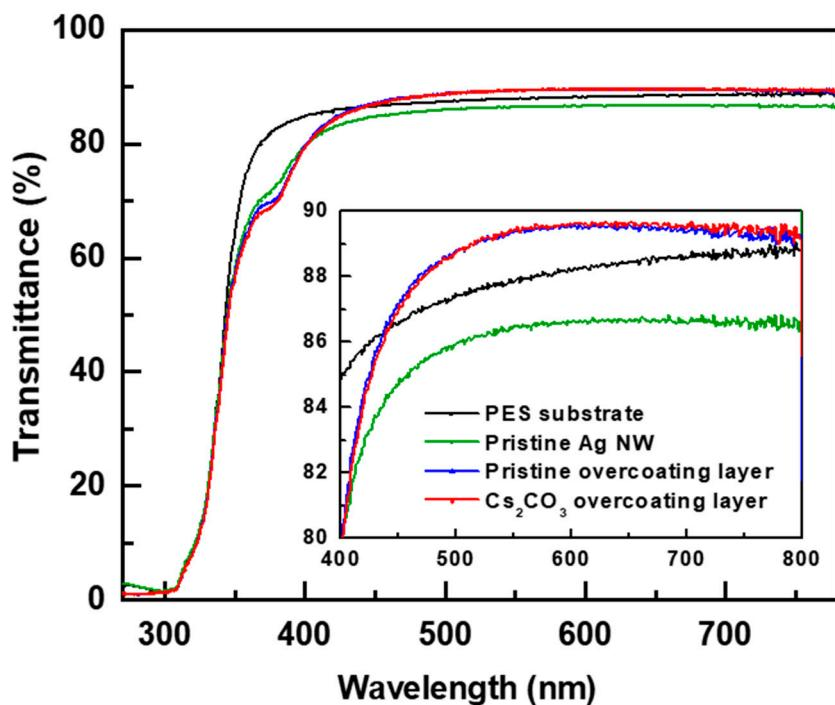
**Figure S2.** Optical transmission spectra of the PES substrate, pristine Ag NWs, Ag NWs covered with the pristine overcoating layer, and Ag NWs covered with the  $\text{Cs}_2\text{CO}_3$ -incorporated overcoating layer. Inset shows the magnified optical transmission spectra of the samples from 80% to 90% transmittance.
