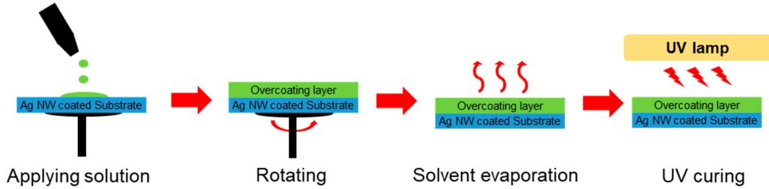
**Figure S1.** Schematic illustration of the steps involved in fabricating the overcoating layer.
