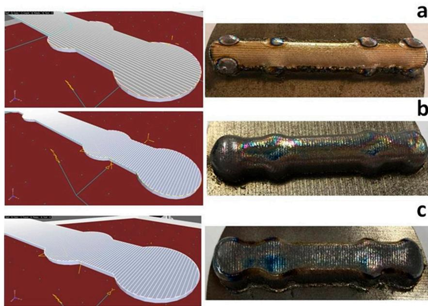
**Figure 12.** Scanning mode during printing and the resulting incipient form: (a) transversal scanning, (b) longitudinal scanning, and (c) longitudinal scanning with the supplemental contour.
