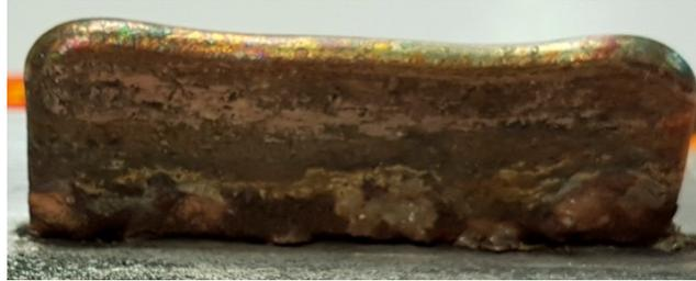
**Figure 4.** Ti6Al4V wall grown by Laser Melting Deposition (LMD).
