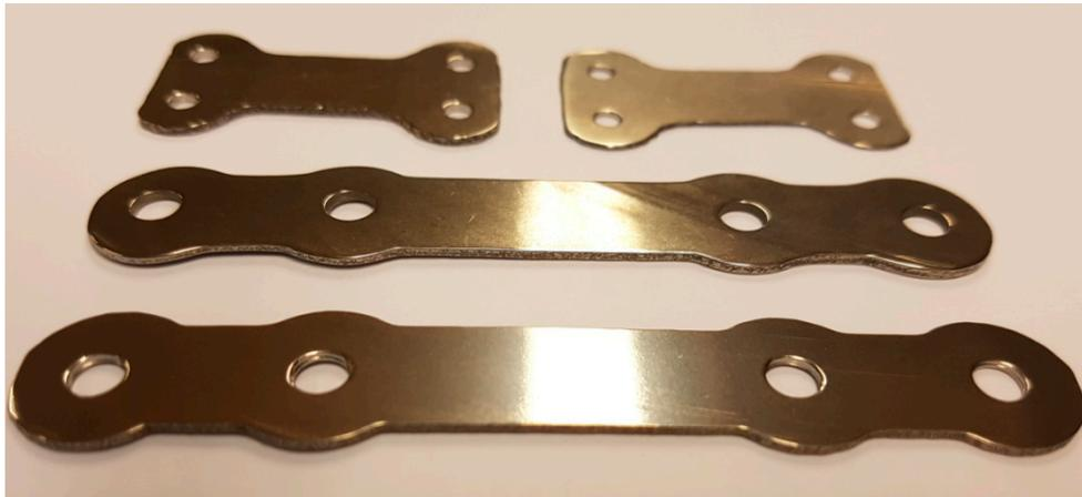
**Figure 15.** Photo of bone plates in the final form produced by Laser Melting Deposition (LMD) and mechanically processed for dimensions and roughness requirements.
