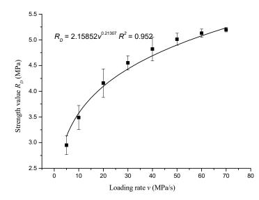
Figure 3. The curve of direct tensile strength of asphalt mixture with loading rate.
