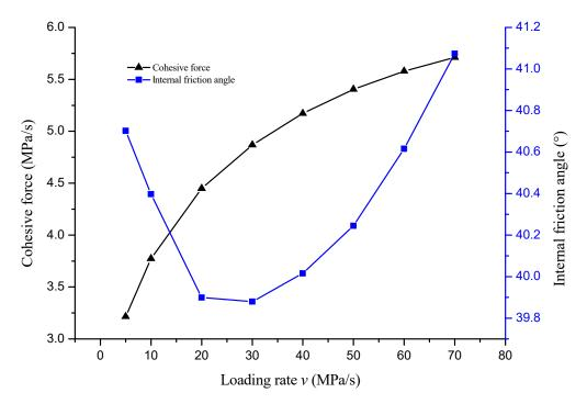
Figure 7. The variation of cohesive force and internal friction angle with loading rate.
