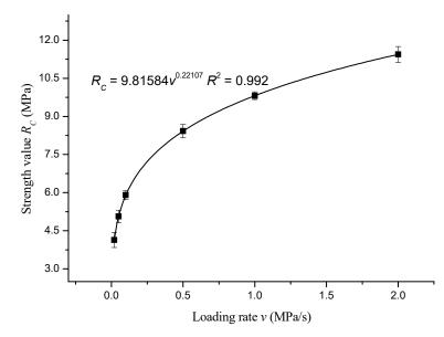
Figure 5. Unconfined compressive strength versus loading rate of asphalt mixture.
