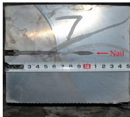
Figure 6. Section morphology of billet after nail shooting. The picture was taken using a digital camera. Adapted from [38].
