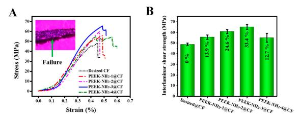
**Figure 7.** (**A**) Stress–strain curves in interlaminar shear strength (ILSS) tests, (**B**) ILSS at different degrees of amination of PEEK.
