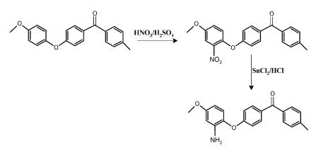
Figure 1. Amination of polyetheretherketone (PEEK).
