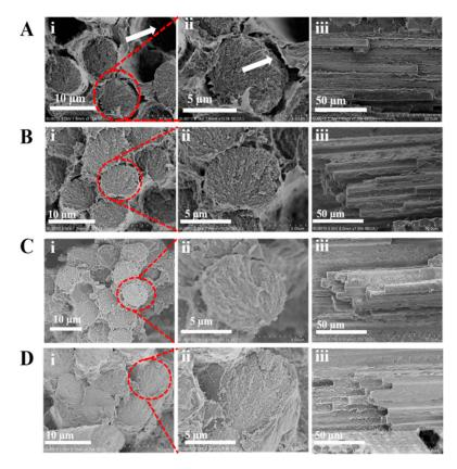
**Figure 9.** SEM images of fracture surface micrographs of CF-PEEK composites containing CF with different modifications: (**A**) Desized@CF, (**B**) PEEK-NH<sub>2</sub>-1@CF, (**C**) PEEK-NH<sub>2</sub>-2@CF, and (**D**) PEEK-NH<sub>2</sub>-3@CF.
