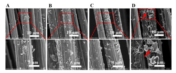
**Figure 3.** SEM images of (**A**) PEEK-NH<sub>2</sub>-1@CF, (**B**) PEEK-NH<sub>2</sub>-2@CF, (**C**) PEEK-NH<sub>2</sub>-3@CF, and (**D**) PEEK-NH<sub>2</sub>-4@CF.
