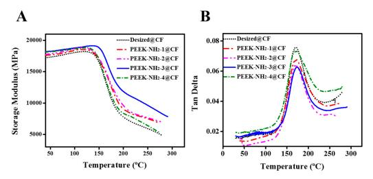
**Figure 8.** (A) Storage modulus and (B) tan  $\delta$  of PEEK-NH<sub>2</sub> modified CF/PEEK composites.
