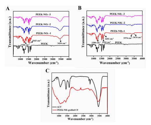
**Figure 6.** FTIR spectra (**A**) nitrided PEEK, (**B**) aminated PEEK, and (**C**) activated-CF (ACF) and PEEK-NH<sub>2</sub> grafted CF.
