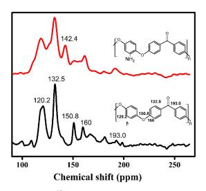
Figure 5. <sup>13</sup>C NMR of PEEK and PEEK-NO<sub>2</sub>.
