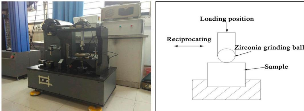
Figure 1. Friction and wear experiment device.
