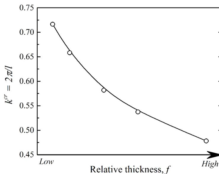
**Figure A1.** Dependence of critical wavenumber on relative thickness of interphasial layer.
