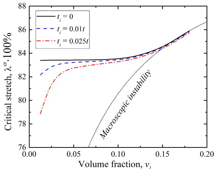
**Figure 7.** Dependence of the critical stretch ratio  $\lambda^{cr}$  on the volume fraction in the layered composite with  $\mu_l/\mu_m = 15$  and shear modulus distribution B. The black dotted curve represents the onset of macroscopic instability in the ideal composites (8).
