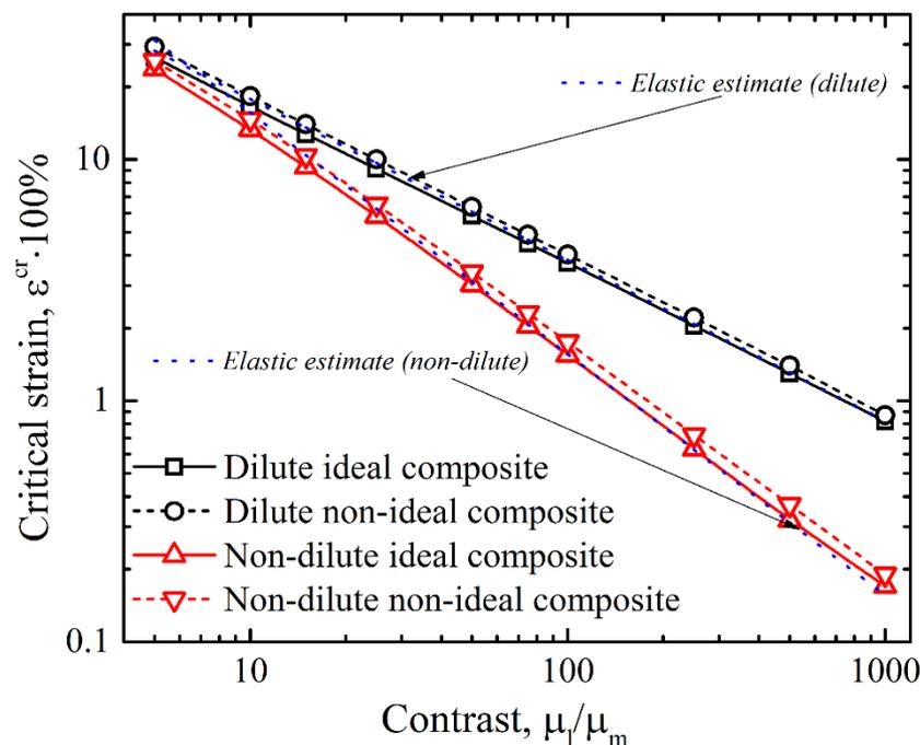
**Figure 4.** The dependencies of critical strain on the contrast in ideal layered composites with  $v_l = 0.025$  (continuous black) and  $v_l = 0.2$  (continuous red) and non-ideal composites with  $v_l = 0.025$  and  $f = 0.5$  (dashed black) and  $v_l = 0.2$  and  $f = 0.5$  (dashed red). Dotted blue curves correspond to the elastic estimates [1,27].
