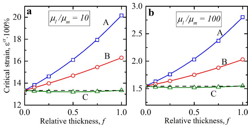
**Figure 5.** Critical strains in the non-dilute composites with interphasial layers. The shear modulus contrast  $\mu_l/\mu_m$  is 10 (a) and 100 (b) and the volume fraction  $v_l = 0.2$ . Horizontal dashed black line corresponds to the case of ideal composites.
