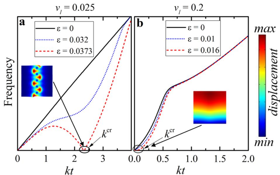
**Figure 3.** The evolution of the dispersion curves of the lowest eigenfrequency during compression of ideal layered composite with  $v_l = 0.025$  (dilute)—(a) and  $v_l = 0.2$  (non-dilute)—(b). The elastic modulus contrast is  $\mu_l/\mu_m = 100$ .
