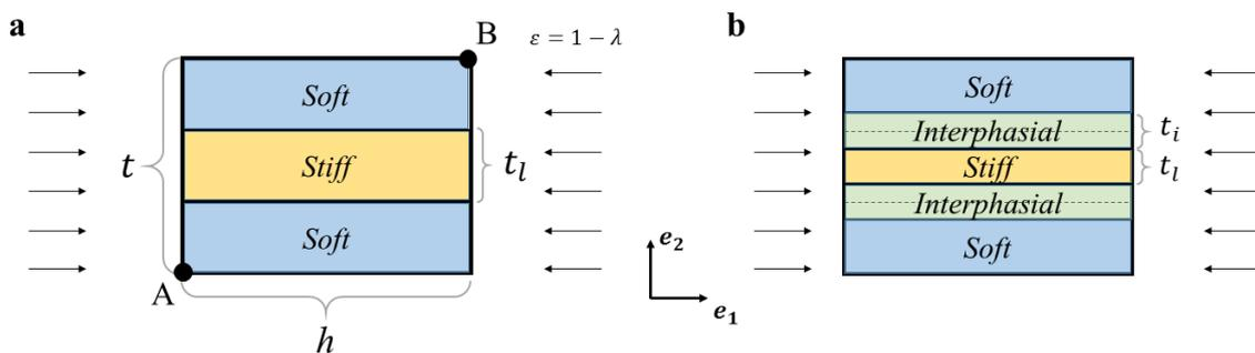
**Figure 1.** Unit cells of “ideal” layered composite (a) and “non-ideal” composite with interphasial layers (b).
