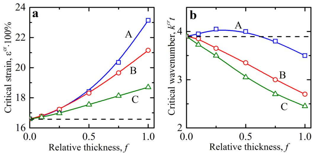
**Figure 6.** Critical strains (a) and wavenumbers (b) in the dilute composites with interphasial layers. The volume fraction is  $v_l = 0.025$ . Horizontal dashed black line corresponds to the case of ideal composites.
