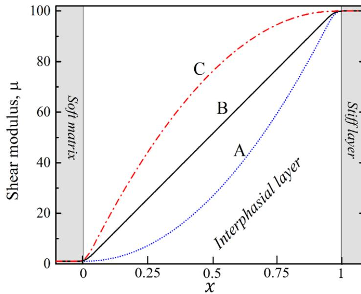
Figure 2. Different types of shear modulus variation in the interphasial layer.
