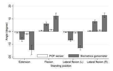
**Figure 3.** Bar chart showing mean angles and standard deviations of flexion, extension and lateral bend of both directions for the POF sensor (white bar chart) and Biometrics goniometer (grey bar chart).
