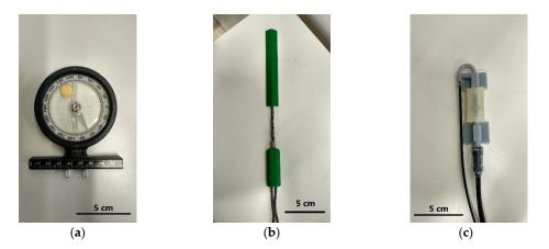
Figure 1. (a) Inclinometer. (b) Biometrics goniometer. (c) Plastic optical fiber (POF) sensor.
