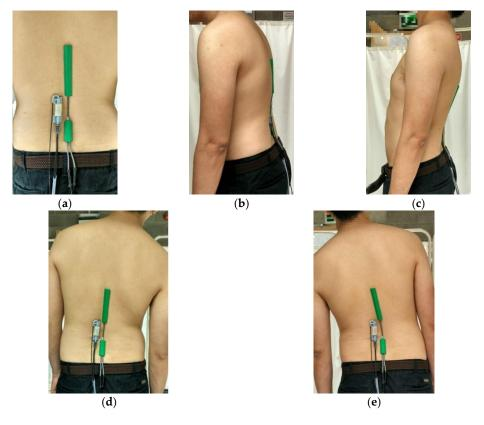
Figure 2. (a) Participant in a reference standing position having the POF sensor and Biometrics goniometer firmly attached next to each other on the skin at the low back-location. (b) Participant in the position for measuring flexion angle. (c) Participant in the position for measuring extension angle. (d) Participant in the position for measuring lateral bend (right) angle. (e) Participant in the position for measuring lateral bend (left) angle.
