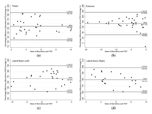
**Figure 5.** Bland–Altman plots between the POF sensor and Biometrics goniometer showing mean and percentage differences with the 95% limits of agreement (LOA) for each movement including (**a**) flexion, (**b**) extension, (**c**) left lateral bend and (**d**) right lateral bend.
