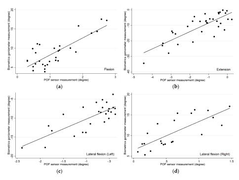
**Figure 4.** Scatter plots showing the linear relationship between the POF sensor and Biometrics goniometer for each movement including (**a**) flexion, (**b**) extension, (**c**) left lateral bend and (**d**) right lateral bend.
