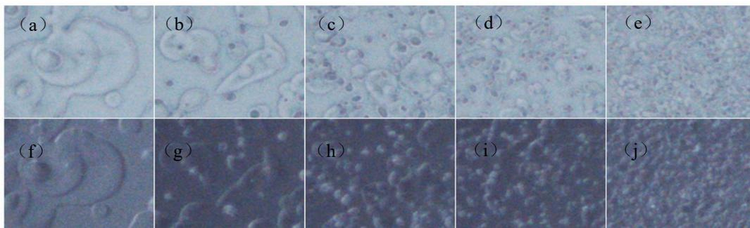
**Figure 6.** The digital microscope pictures of microstructure morphology of anti-glare samples by different air transport pressure (a) 60 kPa (90°); (b) 120 kPa (90°); (c) 210 kPa (90°); (d) 300 kPa (90°); (e) 600 kPa (90°); (f) 60 kPa (25°); (g) 120 kPa (25°); (h) 210 kPa (25°); (i) 300 kPa (25°); and (j) 600 kPa (25°) with the sol-gel deliver pressure and displacement speed of 120 kPa and 300 mm/s, respectively.
