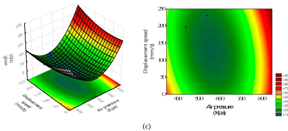
**Figure 9.** The response surface plots of gloss against the factors of (a) sol-gel deliver pressure ( $X_1$ ) and air transport pressure ( $X_2$ ) with  $X_3$  of 140 mm/s; (b) displacement speed ( $X_3$ ) and sol-gel deliver pressure ( $X_1$ ) with  $X_2$  of 560 kPa; and (c) displacement speed ( $X_3$ ) and air transport pressure ( $X_2$ ) with  $X_1$  of 250 kPa.
