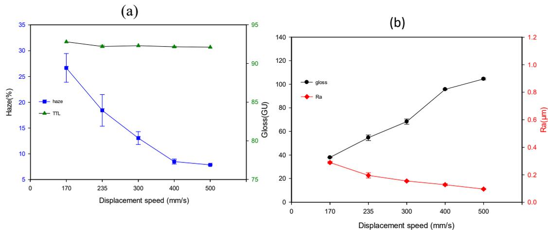
**Figure 7.** The influences of spray displacement speed on (a) haze and TTL, and (b) gloss and Ra with the sol-gel deliver and air transport pressures of 120 kPa and 300 kPa, respectively.
