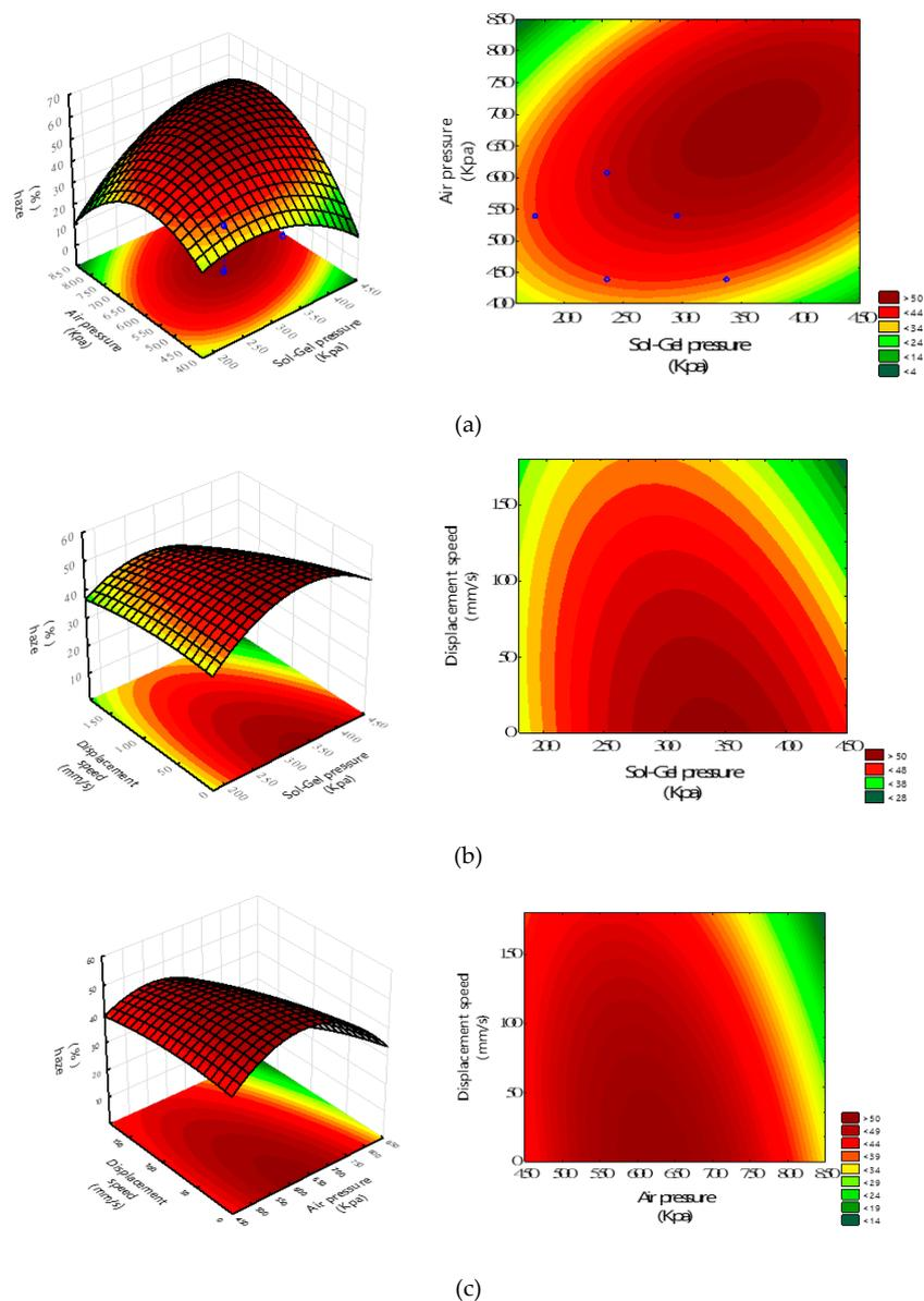
**Figure 10.** The response surface plots of haze against the factors of (a) sol-gel deliver pressure ( $X_1$ ) and air transport pressure ( $X_2$ ) with  $X_3$  of 20 mm/s; (b) displacement speed ( $X_3$ ) and sol-gel deliver pressure ( $X_1$ ) with  $X_2$  of 620 kPa; and (c) displacement speed ( $X_3$ ) and air transport pressure ( $X_2$ ) with  $X_1$  of 340 kPa.
