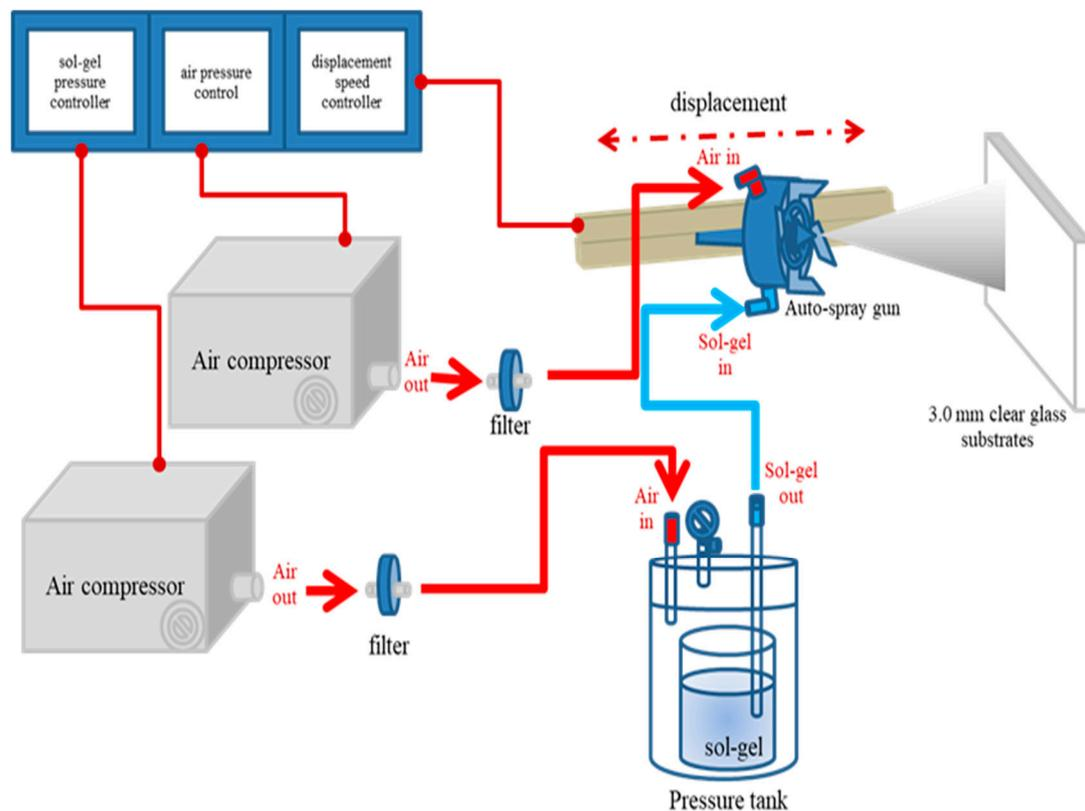
**Figure 2.** Schematic diagram of the anti-glare thin film production by the auto-spray system.
