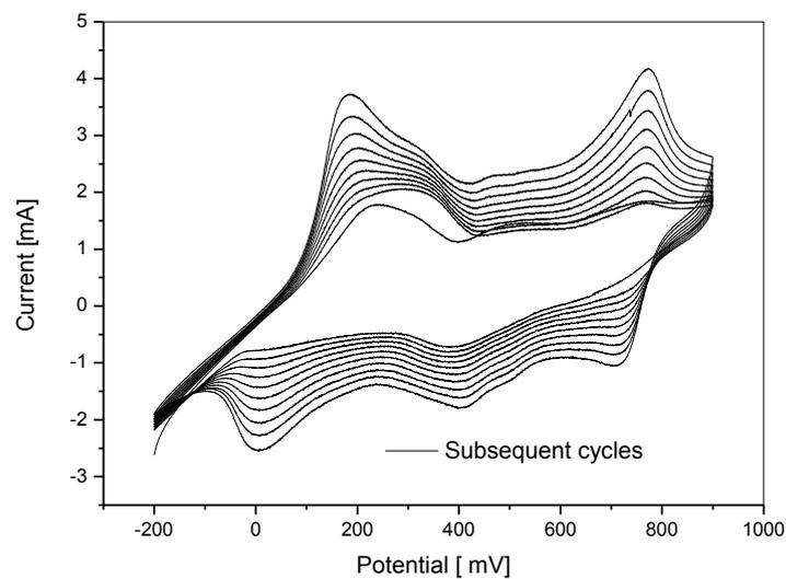
**Figure S2.** Cyclic voltammetry of aniline polymerization on a glassy carbon electrode in 0.1 M aniline + 0.5 M H<sub>2</sub>SO<sub>4</sub> solution at 50 mV/s from -200 to 900 mV for 10 subsequent cycles.
