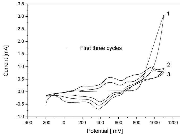
**Figure S1.** Cyclic voltammetry of aniline polymerisation on a glassy carbon electrode in 0.1 M aniline + 0.5M H<sub>2</sub>SO<sub>4</sub> solution at 50 mV/s from -200 to 1100 mV for the first activation cycles.
