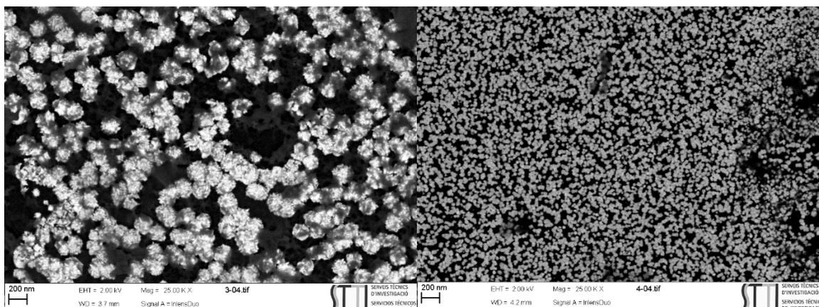
**Figure S5.** SEM micrographs of GC/PANI(CV)/PtNPs obtained with the following deposition conditions:  $E_{on} = -500$  mV (left)  $E_{on} = -750$  mV (right),  $E_{off} = +750$  mV,  $t_{on} = 5$  ms, and DC = 50%. 5 mM  $\text{K}_2\text{PtCl}_6$  in 0.5 M  $\text{H}_2\text{SO}_4$ .
