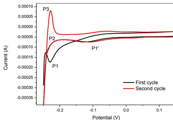
**Figure S3.** Cyclic voltammetry recorded on glassy carbon electrode at 10 mV/s for 5 mM  $\text{K}_2\text{PtCl}_6$  + 0.5 M  $\text{H}_2\text{SO}_4$  plating solution.
