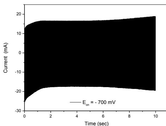
**Figure S4.** Chronoamperometric curve for potentiostatically electrodeposited platinum on GC/ PANI electrodes at a pulse deposition potential  $E_{on} = -700$  mV. Deposition conditions (0.005 M  $\text{K}_2\text{PtCl}_6$  in 0.5 M  $\text{H}_2\text{SO}_4$ ):  $t_{on} = 5$  ms,  $E_{off} = +1$ V,  $t_{dep} = 5$  s, and DC = 50%.
