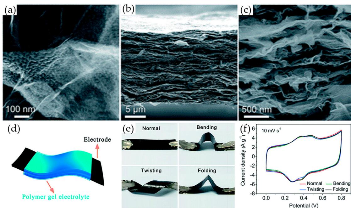
**Figure 13.** (a) SEM images of the 3DG/PANI composite; (b) Low- and (c) high-magnification SEM side view of the flexible 3D-G/PANI composite film; (d) Schematic illustration of a flexible 3D-G/PANI composite-based ASS; (e) Digital photographs of the flexible ASS under normal, bent, twisted and folded states; (f) CV curves of the flexible ASS under different deformation conditions. Reproduced with permission from [134]. The Royal Society of Chemistry (2017).
