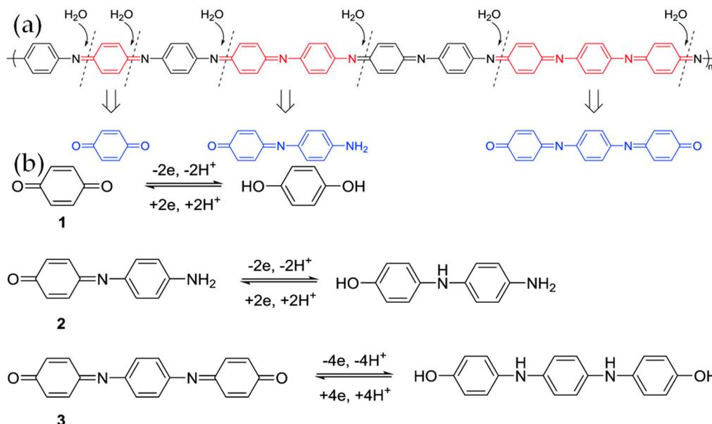
**Figure 5.** (a) Degradation of PANI during the electrochemical process; (b) Reversible redox reaction of HQ and HAOANIs. Reproduced with permission from [56]. The Royal Society of Chemistry (2018).
