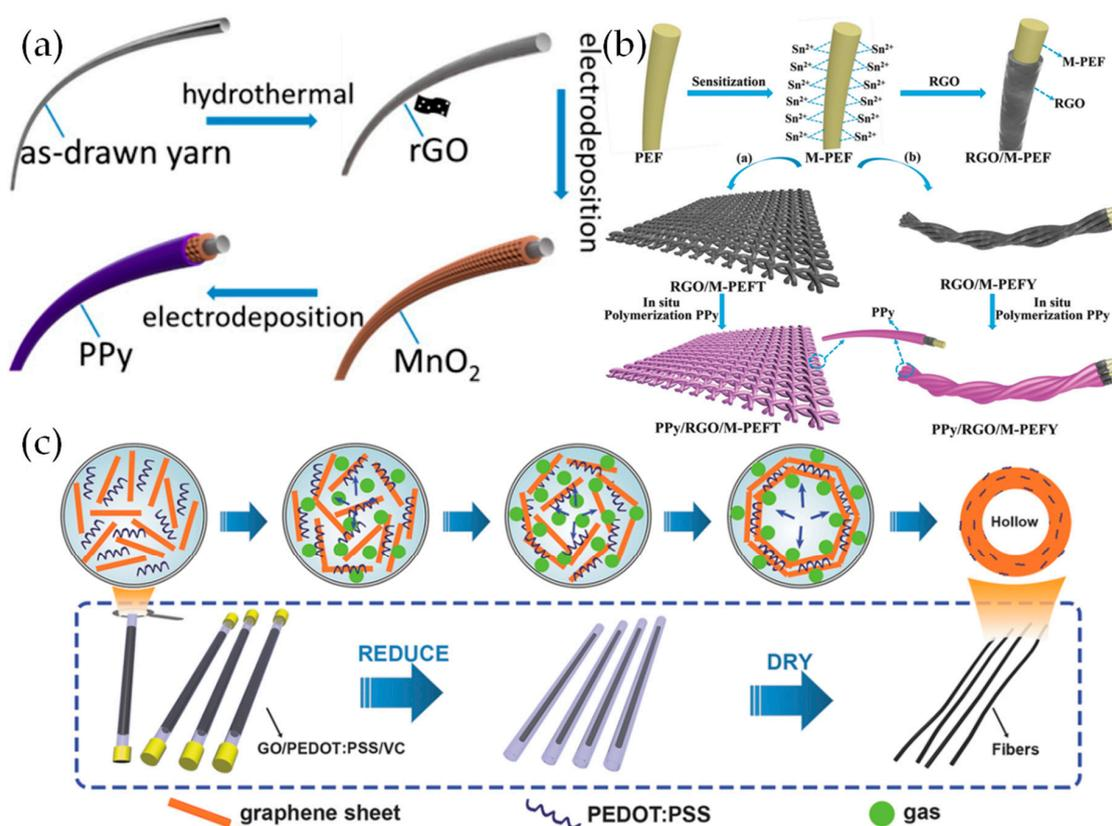
**Figure 15.** (a) Schematic illustration of the yarn modified by deposition of rGO, MnO<sub>2</sub> and PPy. Reproduced with permission from [137]. American Chemical Society (2015). (b) Schematic illustration of the synthesis route toward of textile electrodes and yarn electrodes. Reproduced with permission from [142]. Wiley (2018). (c) The preparation scheme for hollow structure composites. Reproduced with permission from [138]. Wiley (2016).
