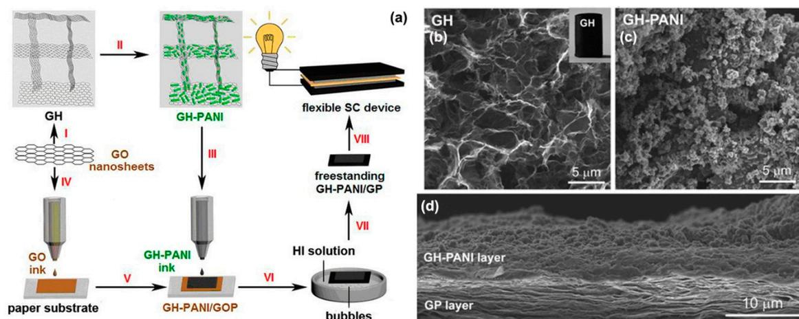
**Figure 12.** (a) Schematic illustration of the fabrication process of GH PANI/GP; SEM images of GH (b); GH-PANI (c); GH-PANI/GP (d). Reproduced with permission from [133]. American Chemical Society (2014).
