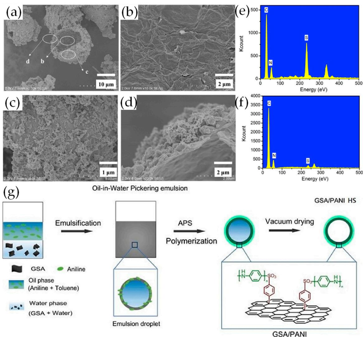
**Figure 3.** (a) GSA/PANI HS FE-SEM images of; FE-SEM images of (b) inner wall, (c) outer wall and (d) edge of GSA/PANI HS; (e) EDX spectrum of the regions of GSA/PANI HS inner wall; (f) EDX spectrum of the regions of GSA/PANI HS outer wall; (g) Schematic illustration of the fabrication of GSA/PANI HS via Pickering emulsion route; Reproduced with permission from [53]. Elsevier (2018).
