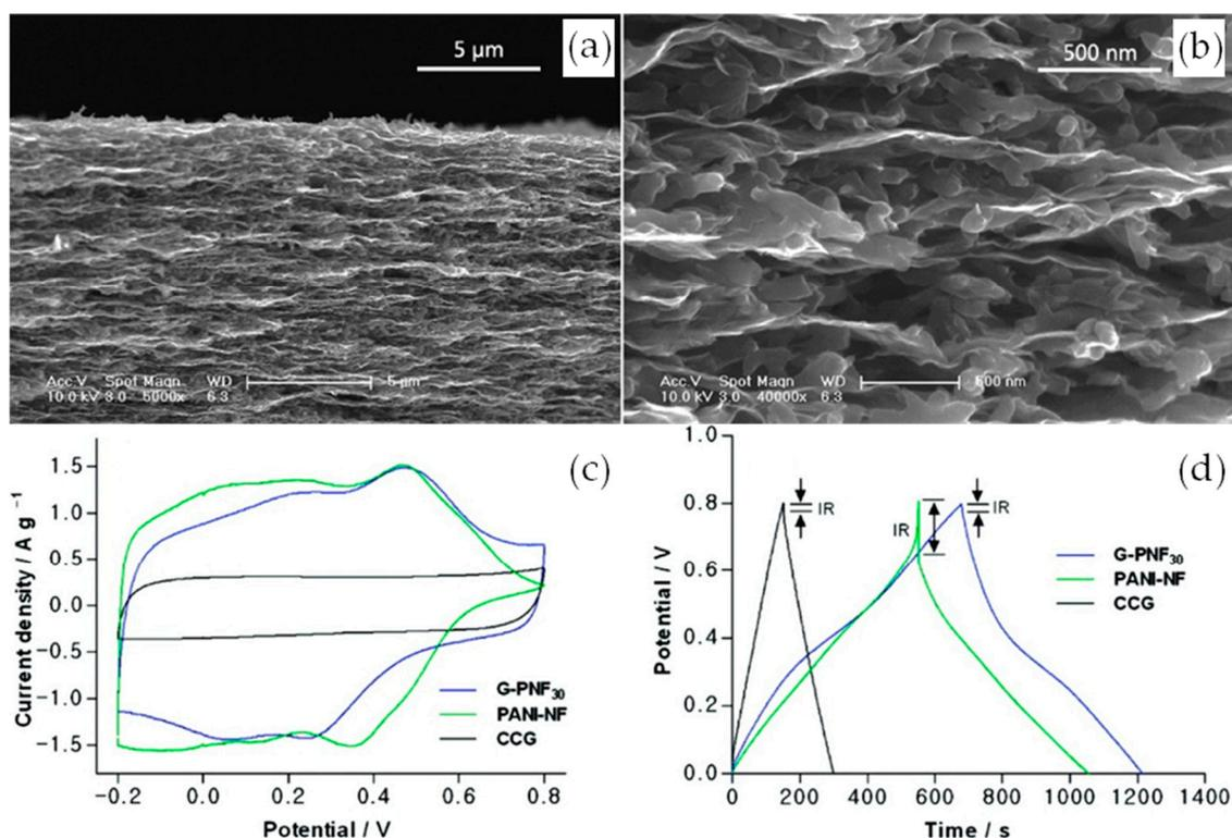
**Figure 1.** (a,b) Cross-sectional SEM images of G-PNF<sub>30</sub>; (c) CV curves of supercapacitors based on G-PNF<sub>30</sub>, as-formed PANI-NF, and CCG films; (d) GCD curves of the supercapacitors based on G-PNF<sub>30</sub>, as-formed PANI-NF, and CCG films. Reproduced with permission from [47]. American Chemical Society (2010).
