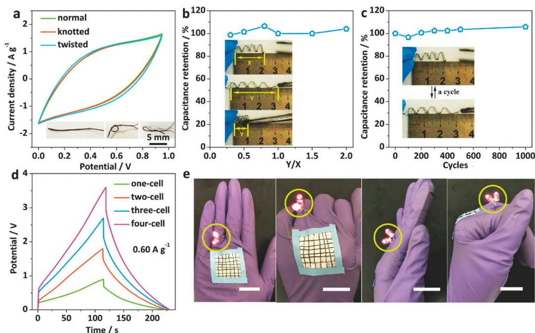
**Figure 16.** (a) CV curves of the assembled all-hydrogel-state cell in different states; (b,c) the elasticity of the spring-like full cell; (d) several full cells connected in series; (e) a demonstration of yarn powering two LEDs in the normal and curved states. Reproduced with permission from [143]. Wiley (2018).
