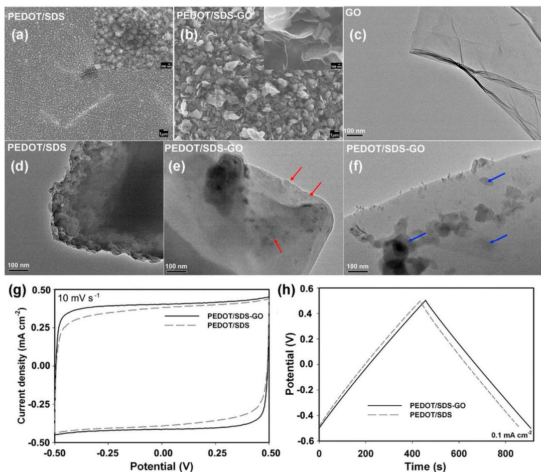
**Figure 8.** SEM images of PEDOT/SDS (a) and PEDOT/SDS-GO (b) composite films; TEM images of GO (c), PEDOT/SDS (d), and PEDOT/SDS-GO composites (e), (f). Reproduced with permission from [86]. Elsevier (2018).
