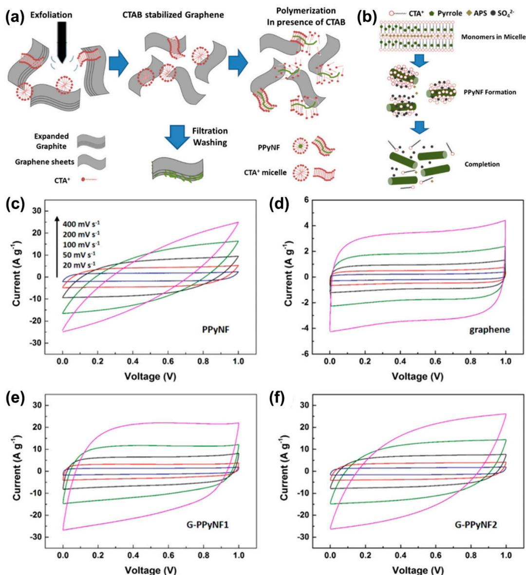
**Figure 6.** (a) The preparation scheme of G-PPyNF film; (b) Schematic illustration of the formation of PPyNF; CV curves of PPyNF (c), graphene (d), G-PPyNF1 (e), and G-PPyNF2 (f) electrodes. Reproduced with permission from [63]. American Chemical Society (2018).
