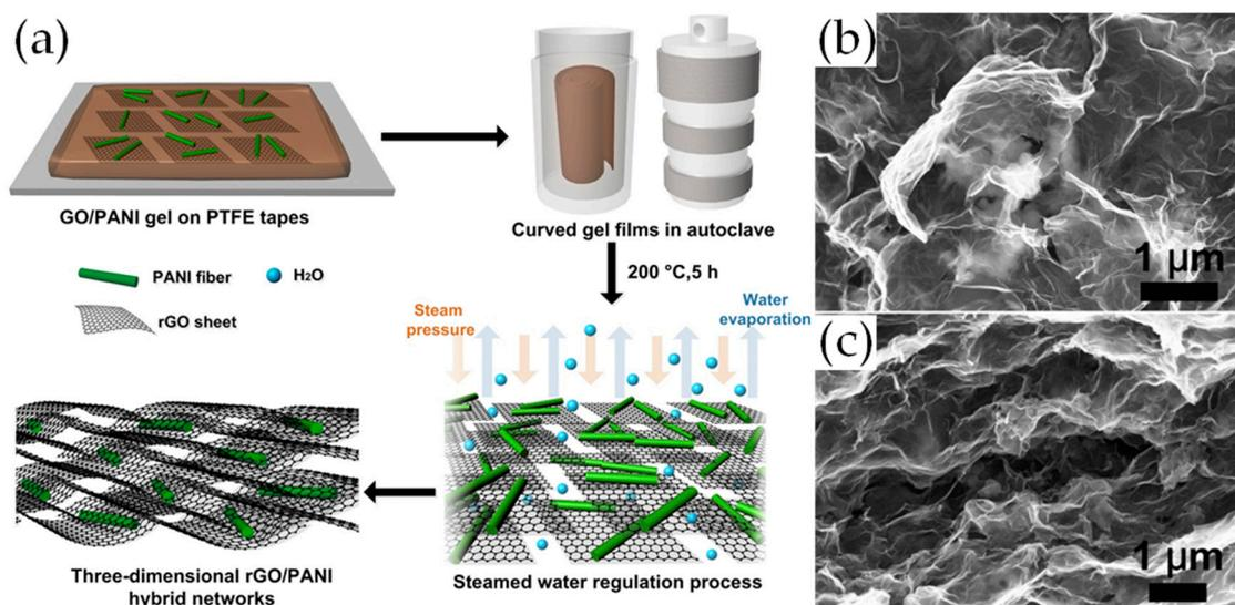
**Figure 4.** (a) Schematic illustration of rGO/PANI hybrid films by steamed water regulation techniques; (b) FE-SEM images of rGO/PANI (50%) hybrid films; (c) Cross-section FE-SEM images of rGO/PANI (50%) hybrid films. Reproduced with permission from [54]. Elsevier (2017).
