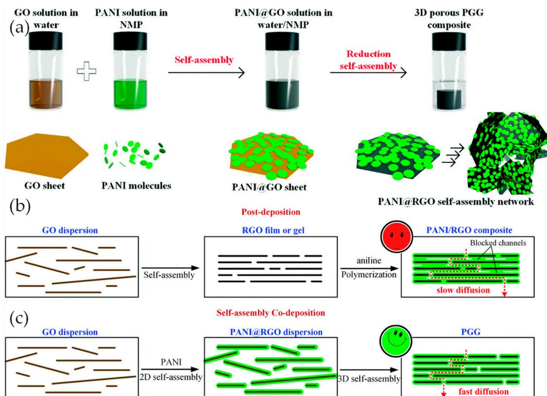
**Figure 2.** (a) Schematic illustration of the solution-based self-assembly method for the preparation of PGGs; (b) Schematic illustration of the formation of partially blocked channels in in situ polymerization of aniline on an RGO matrix; (c) Schematic illustration of the formation of unblocked channels in a self-assembly process. Reproduced with permission from [48]. The Royal Society of Chemistry (2018).
