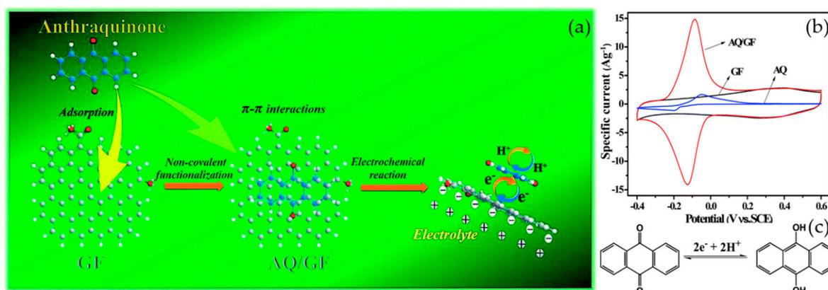
**Figure 10.** (a) Schematic illustration of AQ/GF composite; (b) CV curves of AQ, GF and AQ/GF; (c) The corresponding redox reactions by a coupled proton–electron transfer. Reproduced with permission from [104]. The Royal Society of Chemistry (2015).
