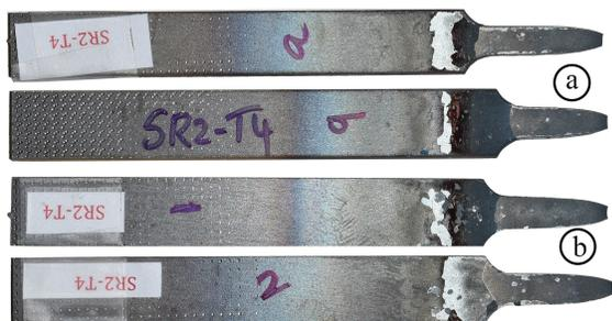
(a) Fractured specimens at 950 °C and 0.1 s<sup>-1</sup>
