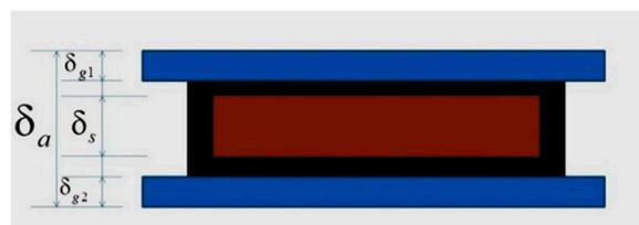
**Figure 8.** Schematic of asphalt film thickness measurement.
