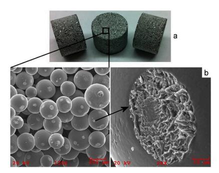
**Figure 6.** Porous Ti5Al2.5Fe compacts (**a**), contacts between the particles showing dimpled fracture surface (**b**). Reprinted from Yamanoglu et al. [24], Copyright (2016), with permission from Elsevier.
