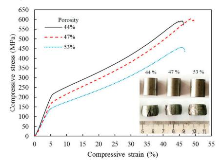
**Figure 17.** Room temperature uniaxial compressive stress–strain curves of porous iron prepared by pressureless SPS from the pre-compacted iron nitride powder. Reprinted from Cui et al. [40], Copyright (2016) by the authors; this article is an open access article distributed under the terms and conditions of the Creative Commons Attribution (CC-BY) license (http://creativecommons.org/licenses/by/4.0/).
