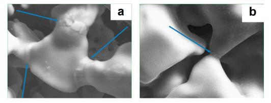
**Figure 7.** Inter-particle necks formed between  $V_8C_7$  particles: (a) free pressureless SPS at 1550 °C, holding time 40 min, (b) conventional sintering at 1550 °C, holding time 180 min. Reprinted from Giuntini et al. [23], Copyright (2013), with permission from Elsevier.
