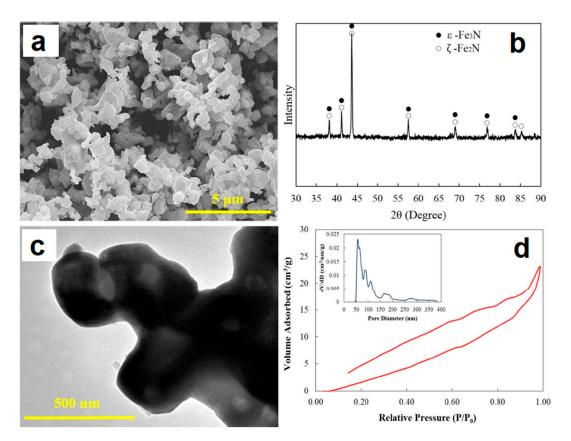
**Figure 15.** Morphology (**a**), X-ray diffraction (XRD) pattern (**b**), structure in the transmission electron microscope (**c**) and adsorption–desorption isotherm/pore size distribution (**d**) of the iron nitride-based powder. Reprinted from Cui et al. [40], Copyright (2016) by the authors; this article is an open access article distributed under the terms and conditions of the Creative Commons Attribution (CC-BY) license (http://creativecommons.org/licenses/by/4.0/).
