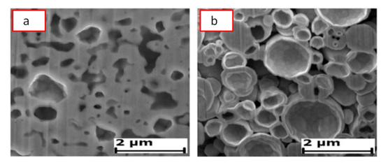
**Figure 11.** Cross-section of porous nickel obtained by pressureless SPS of hollow Ni particles obtained by spray solution combustion synthesis: (**a**) 500 °C, 30 min, porosity 70%; (**b**) 500 °C, 15 min, porosity 88%. Reprinted from Trusov et al. [22], Copyright (2018), with permission from Elsevier.
