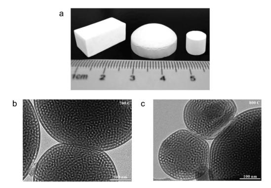
**Figure 9.** Meso/macroporous silica compacts obtained by SPS at 700 °C and 20 MPa from an amorphous silica powder (**a**), transmission electron microscopy images of the contacts between porous silica particles formed in the compacts subjected to SPS at 700 °C (**b**) and 800 °C (**c**) and a pressure of 20 MPa. Reprinted from Vasiliev et al. [60], Copyright (2006), with permission from the American Chemical Society.
