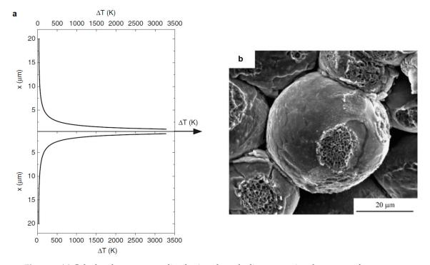
**Figure 3.** (a) Calculated temperature distribution along the line connecting the centers of two copper particles (the current passing through the sample was 1000 A, the sample diameter was 20 mm, the copper particle diameter was 20  $\mu$ m), (b) the morphology of the fractured neck between the copper particles (SPS at 660 °C, 20 MPa, the relative density of the sample was 80.1%). Reprinted from Song et al. [29], Copyright (2005), with permission of John Wiley & Sons.
