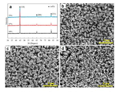
**Figure 16.** XRD patterns (**a**) and structure of porous iron (**b**–**d**) prepared by pressureless SPS from the pre-compacted iron nitride powder ((**b**) porosity 44%, (**c**) 47%, and (**d**) 53%). Reprinted from Cui et al. [40], Copyright (2016) by the authors; this article is an open access article distributed under the terms and conditions of the Creative Commons Attribution (CC-BY) license (http://creativecommons. org/licenses/by/4.0/).
