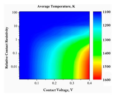
**Figure 4.** Parametric isolines of the average temperature obtained by modeling of resistance heating of spherical copper particles 10 µm in diameter covered with oxide films. Reprinted from Olevsky & Dudina [15], Copyright (2018), with permission of Springer Nature.
