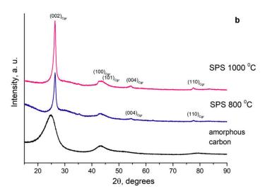
**Figure 22.** XRD patterns of compacts obtained by SPS of the ball-milled Co-17 wt %C mixture at 800 and 1000 °C (**a**), XRD patterns of the starting amorphous carbon (carbon black) and porous graphitized materials obtained by selective dissolution of cobalt from the sintered compacts (**b**). Reprinted from Bokhonov et al. [78], Copyright (2018), with permission from Elsevier.
