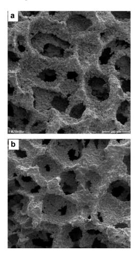
**Figure 21.** Porous structure of Ti6Al4V obtained by SPS with NaCl as a space holder: SPS at 700 °C, 50 MPa and removal of NaCl (**a**), after heat treatment of the porous compact at 1100 °C by pressureless SPS (**b**). Reprinted from Quan et al. [52]. Copyright (2012), with permission from Elsevier.
