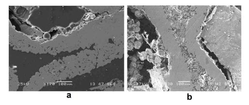
**Figure 13.** Structure of the cell walls of the steel sphere samples after treatment by SPS at 1000  $^{\circ}$ C (a) and 1200  $^{\circ}$ C (b). Reprinted from Khor et al. [55], Copyright (2003), with permission from Elsevier.
