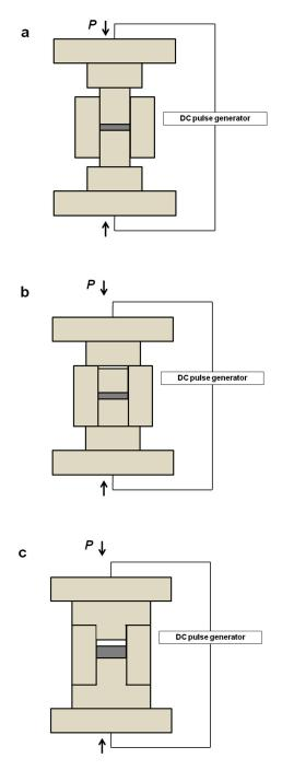
Figure 2. Tooling for pressure-assisted (a) and pressureless SPS ((b) [20-22], (c) [23,24]).
