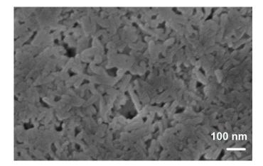
**Figure 20.** Surface of the partially densified hydroxyapatite sample perpendicular to the direction of applied load, SPS temperature 150 °C. Reprinted from Ortali et al. [58], Copyright (2017), with permission from Elsevier.
