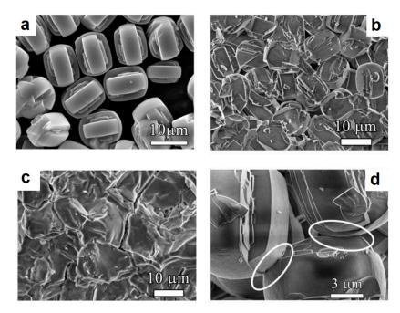
**Figure 8.** Morphology of silicalite-1 particles (**a**), fracture surface of compacts produces by SPS at 1100 °C (**b**,**d**—different magnifications) and 1300 °C (**c**). Reprinted from Vasiliev et al. [63], Copyright (2010) with permission from the American Chemical Society.
