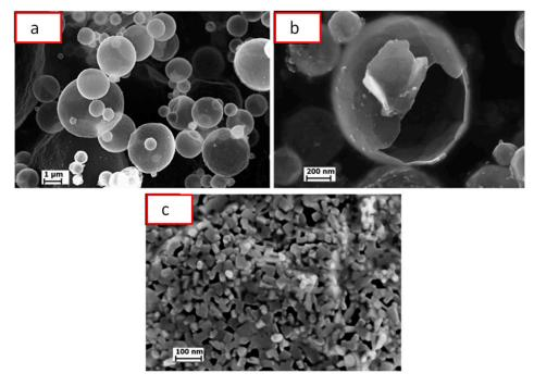
**Figure 10.** Morphology (**a**,**b**) and wall structure (**c**) of hollow Ni particles obtained by spray solution combustion synthesis. Reprinted from Trusov et al. [22], Copyright (2018), with permission from Elsevier.
