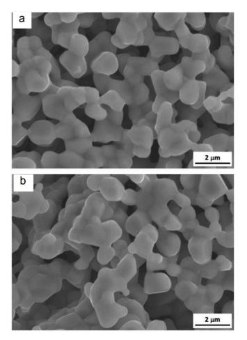
**Figure 19.** Surface of  $ZrB_2$  porous compacts synthesized at 1600 °C, holding time 10 min (**a**), 20 min (**b**). Reprinted from Yuan et al. [66], Copyright (2012), with permission from Elsevier.
