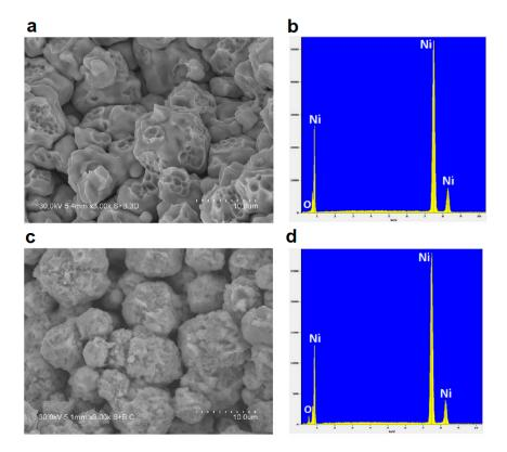
**Figure 5.** Fracture surface (**a**,**c**) and results of the energy-dispersive spectroscopy analysis (**b**,**d**) of nickel compacts consolidated by SPS from a partially oxidized nickel powder, (**a**,**b**) SPS in contact with graphite foil, (**c**,**d**) SPS in contact with copper foil. Reprinted from Dudina & Bokhonov [25], Copyright (2016), with permission from Elsevier.
