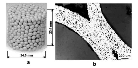
**Figure 12.** General view of the randomly packed steel sphere sample (**a**), porous structure of the cell wall (**b**). Reprinted from Khor et al. [55], Copyright (2003), with permission from Elsevier.
