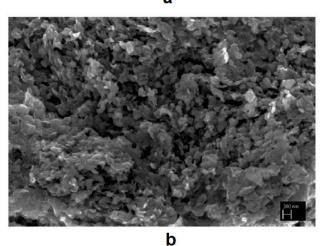
**Figure 23.** Fracture surface of the compact obtained by SPS of the ball-milled Co-17 wt %C mixture at 800 °C (**a**) and the porous graphitized material obtained by selective dissolution of cobalt from the sintered compact (**b**). Reprinted from Bokhonov et al. [78], Copyright (2018), with permission from Elsevier.
