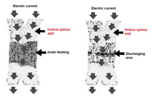
**Figure 14.** Densification of the wall of steel spheres by SPS. Reprinted from Khor et al. [55], Copyright (2003), with permission from Elsevier.
