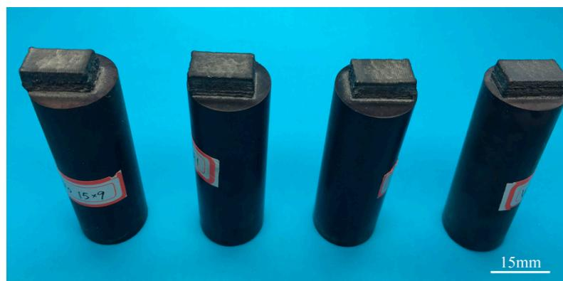
**Figure 3.** Macroscopic photograph of the W<sub>x</sub>NbMoTa alloys.
