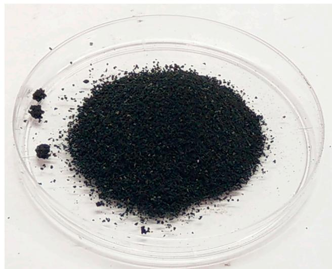
**Figure 1.** As-received crumb rubber.
