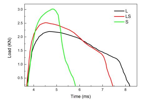
Figure 1. Charpy impact test curves of impact load-time of the samples.
