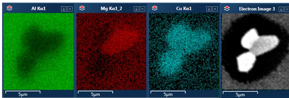
**Figure 8.** Precipitates of  $\text{Al}_2\text{Cu}$  and  $\text{Al}_2\text{CuMg}$  phases found in alloy A.
