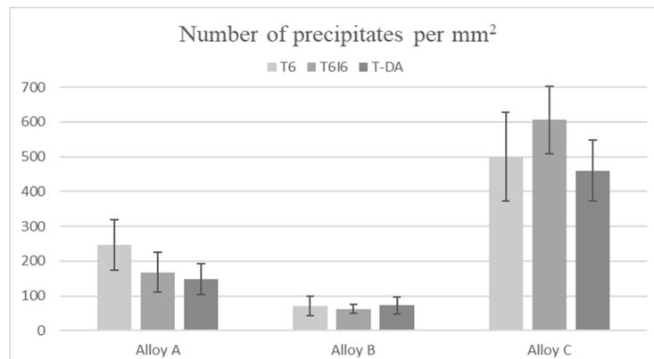
**Figure 4.** Number of precipitates on the examined surface of the specimen per mm<sup>2</sup>.
