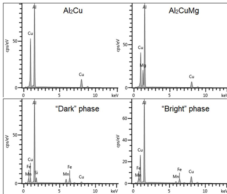
**Figure 6.** Spectra from EDS analysis of the most common phases found in the alloys A, B and C.
