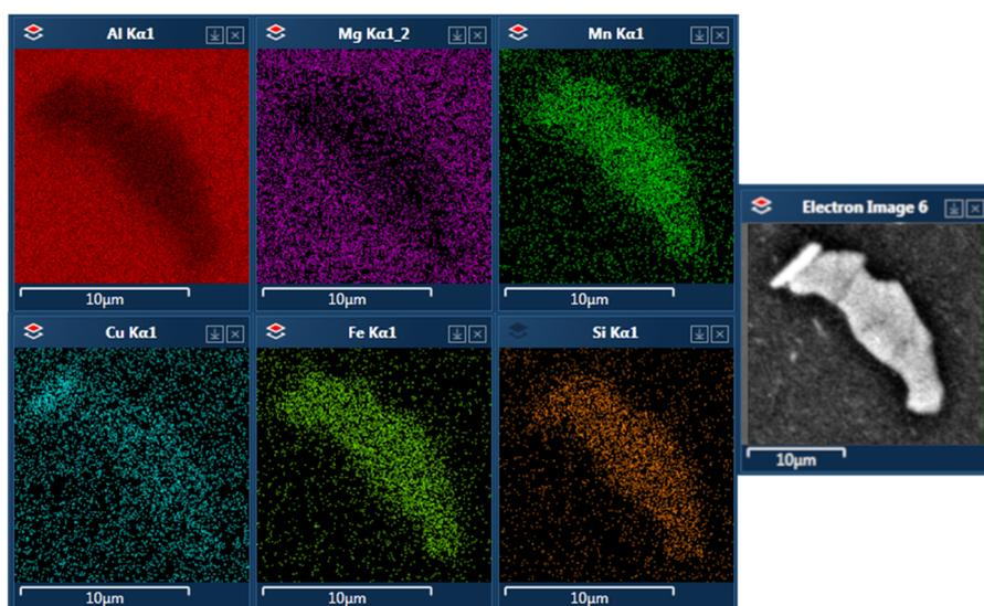
**Figure 7.** A precipitate found in the alloy A after T-DA aging.
