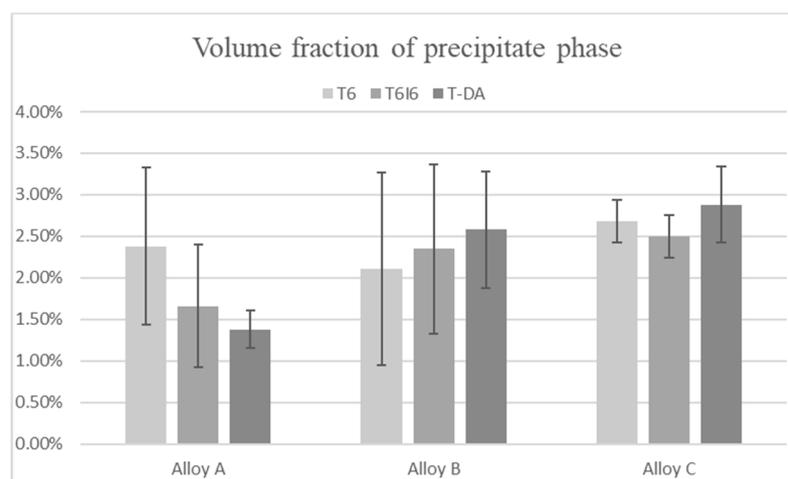
**Figure 3.** Total volume fractions of precipitate phases for all the alloy treatment variants.
