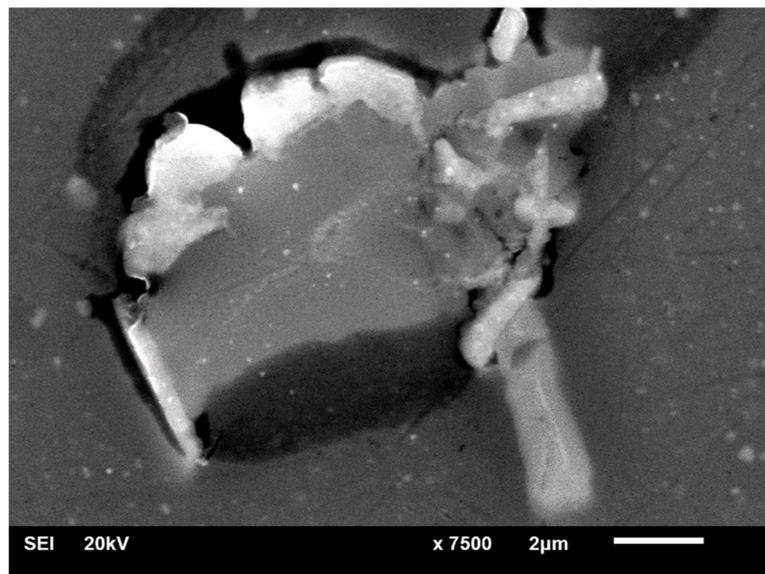
**Figure 10.** A closer view at the multiphase precipitate found in alloy B after T6I6 aging showing the distinction between “bright” and “dark” phases.
