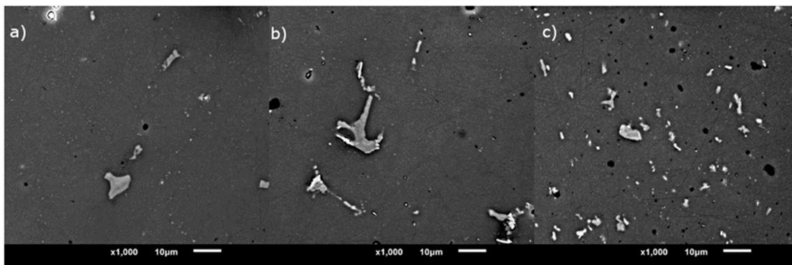
**Figure 2.** Comparison of microstructures of (a) alloy A, (b) alloy B, and (c) alloy C after T6 aging.
