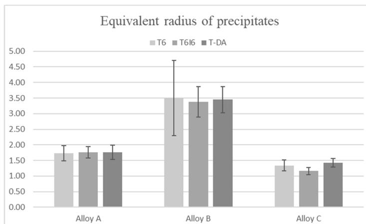
**Figure 5.** The equivalent radius of precipitates on the examined surface of the specimen.
