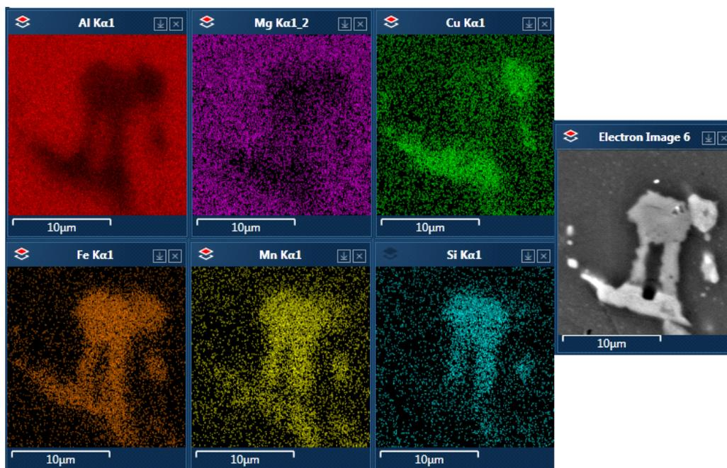
**Figure 9.** A precipitate found in alloy B after T-DA aging.
