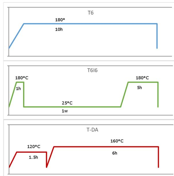
**Figure 1.** Schematic representation of three different aging treatments applied to the examined alloys.
