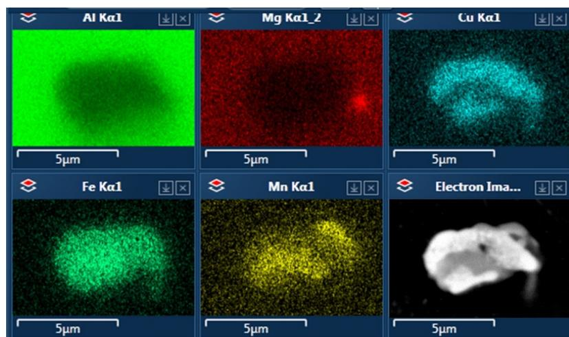
**Figure 11.** A precipitate of core–shell morphology found in alloy C after T6 aging. The results of EDS analysis show differentiation of chemical composition between the two phases.
