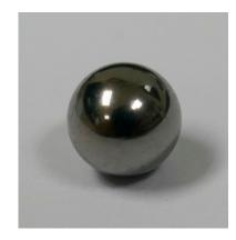
Figure 9. Steel sphere used in calibration.
