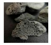
Figure 1. Appearance of lightweight expanded shale aggregates.
