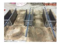
Figure 11. Mold of the beam specimen.
