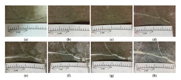
**Figure 17.** Images of the pre-cracked concrete beam specimen with small cracks (Experimental group II): (a) Day 1; (b) Day 3; (c) Day 7; (d) Day 14; (e) Day 21; (f) Day 28; (g) Day 56; (h) Day 91.
