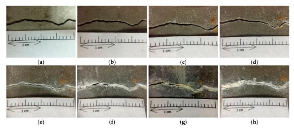
**Figure 18.** Images of the pre-cracked concrete beam specimen with large cracks (Experimental group II): (a) Day 1; (b) Day 3; (c) Day 7; (d) Day 14; (e) Day 21; (f) Day 28; (g) Day 56; (h) Day 91.
