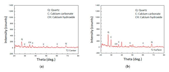
**Figure 25.** XRD test results of the crack repair powder (experimental group II): (**a**) result at the sample center; (**b**) result at the sample surface.
