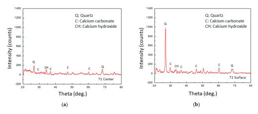
**Figure 24.** XRD test results of crack repair powder (experimental group I): (**a**) result at the sample center; (**b**) result at the sample surface.
