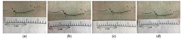
**Figure 13.** Images of the pre-cracked concrete cylindrical specimen (Control group): (**a**) Day 1; (**b**) Day 28; (**c**) Day 56; (**d**) Day 91.
