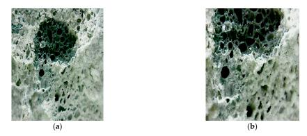
**Figure 20.** Sectional observation of experimental group II under a portable microscope: (**a**) 100 times magnification; (**b**) 200 times magnification.
