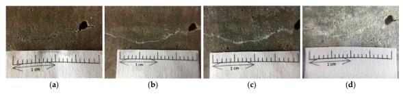
**Figure 15.** Images of the pre-cracked concrete cylindrical specimen (Experimental group II): (**a**) Day 1; (**b**) Day 28; (**c**) Day 56; (**d**) Day 91.
