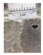
Figure 21. Surface crack of the concrete specimen.
