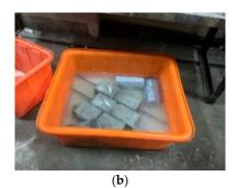
**Figure 3.** Curing situation of specimens: (**a**) control group and experimental group I; (**b**) experimental group II.
