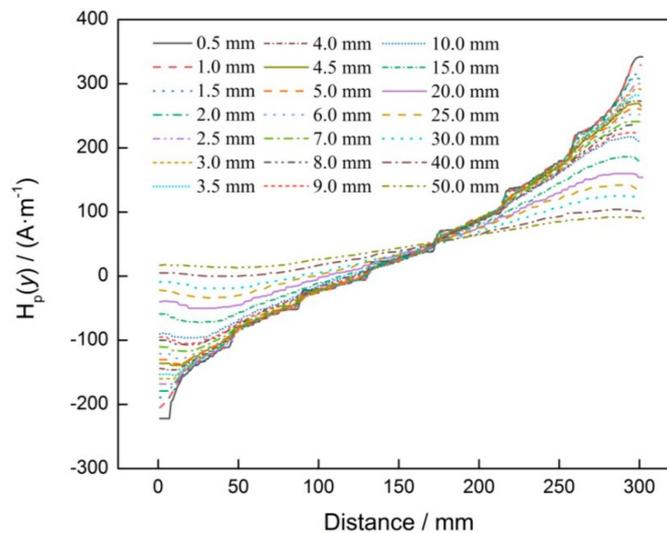
Figure 3.  $H_p(y)$  signal corresponding to different lift-offs of sensor probe.
