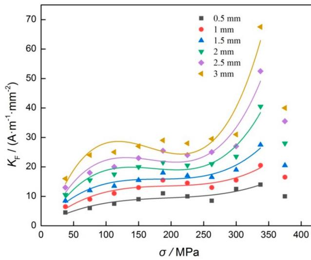
Figure 8. Result of  $K_F$  and tensile stress.
