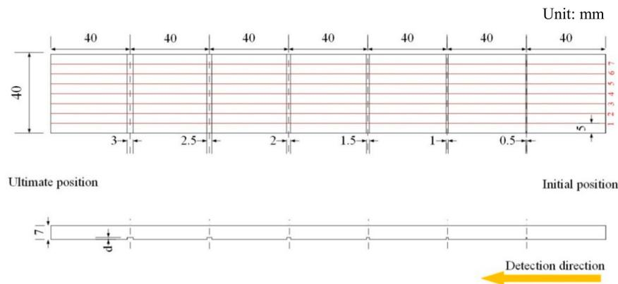
**Figure 1.** The sketch map of the experimental sample with regular rectangular groove.
