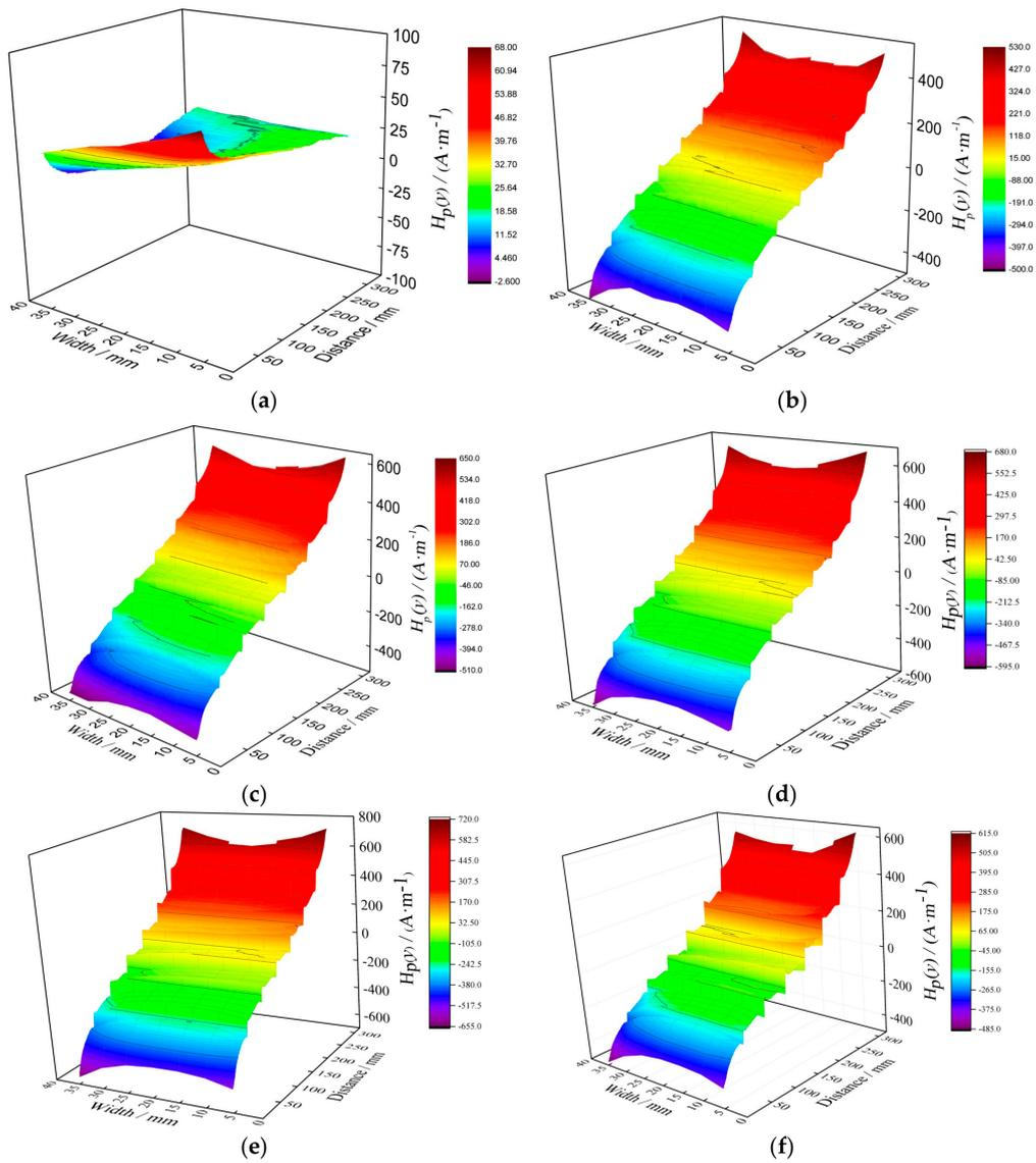
**Figure 4.**  $H_p(y)$  signals under different tensile loads. (a) 0 MPa, (b) 75 MPa, (c) 150 MPa, (d) 225 MPa, (e) 337.5 MPa, (f) 375 MPa.
