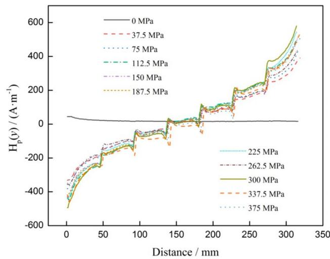
**Figure 5.**  $H_p(y)$  signals corresponding to different stresses.
