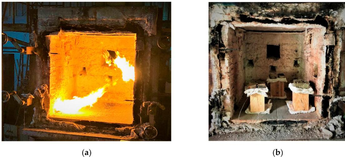
Figure 7. (a) location of fire; (b) arrangement of test specimens.
