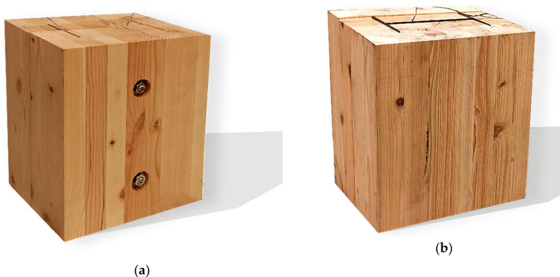
**Figure 5.** TSC specimens: (a) dowel connection and (b) glue connection.
