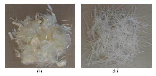
**Figure 1.** Appearance of fibers: (**a**) Polyvinyl alcohol fibers (PVAF); (**b**) Polypropylene plastic steel fibers (PPSF).
