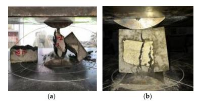
Figure 8. Failure form of specimens in split tensile test: (a) Reference concrete; (b) HFRC.
