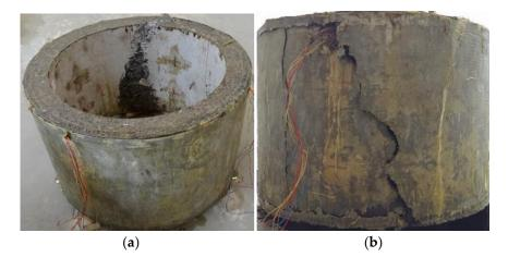
**Figure 9.** Failure characteristic of D-0 model specimen (reference concrete): (**a**) failure characteristic of inside surface (**b**) failure characteristic of outside surface.
