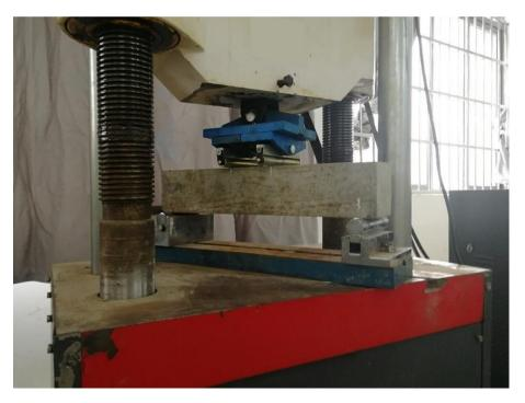
Figure 4. Flexural test.
