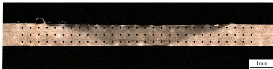
Figure 1. Optical microscope image of the hardness testing point distribution diagram.
