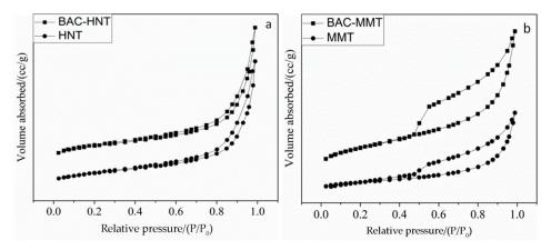
Figure 6. Adsorption–desorption isotherms of (a) HNT- and (b) MMT-loaded BAC before and after.
