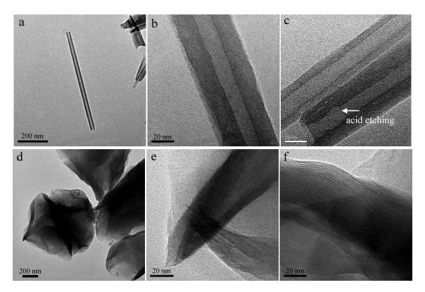
Figure 2. TEM images of (a,b) HNT, BAC-HNT (c), (d,e) MMT, and (f) BAC-MMT.
