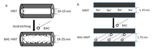
**Figure 1.** The schematics of **(a)** halloysite nanotubes (HNT) and **(b)** montmorillonite (MMT) loading benzyl ammonium chloride (BAC).
