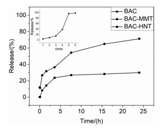
Figure 7. The release profiles of BAC from HNT and MMT.
