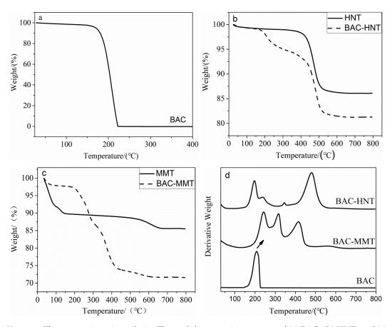
**Figure 3.** Thermogravimetric analysis: Thermal decomposition curves of **(a)** BAC, **(b)** HNT, and **(c)** MMT; **(d)** derivative thermal curves.
