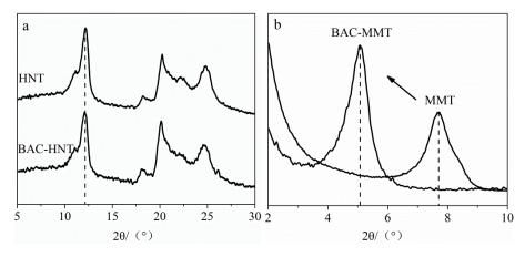
Figure 5. XRD patterns of (a) HNT- and (b) MMT-loaded BAC before and after.
