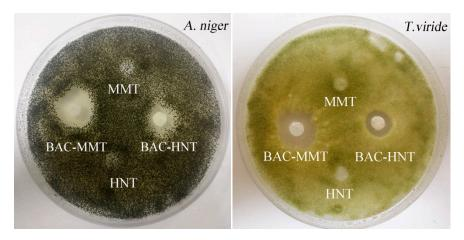
Figure 8. Inhibition zones of BAC-HNT and BAC-MMT against A. niger and T. viride.
