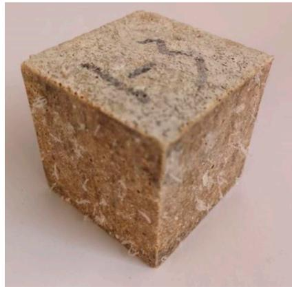
Figure 7. MPC mortar specimen of 7 days immersion.
