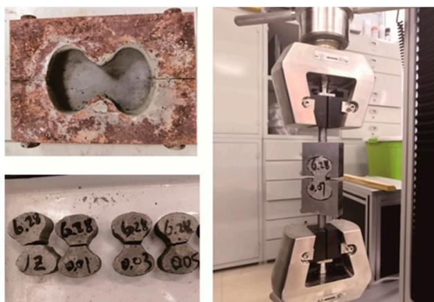
Figure 1. Eight-shaped mold and test method for tensile strength.
