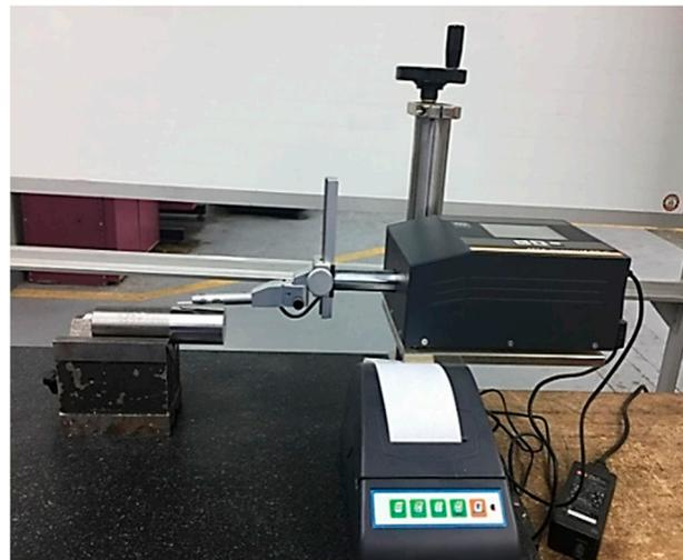
Figure 2. The surface roughness measurements.
