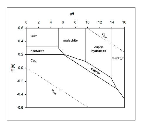
**Figure S4.** Pourbaix diagram of the corrosion by-products formed on the metallic surface of a copperchlorine-carbonate system at 25 °C (respect to SHE). Concentrations increased 10<sup>3</sup> times in order to simulate high availability of hydrogen ion, chloride, and dissolved inorganic carbon at the metalliquid interface.
