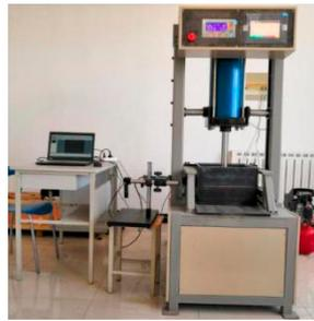
Figure 2. The pull-out test equipment.
