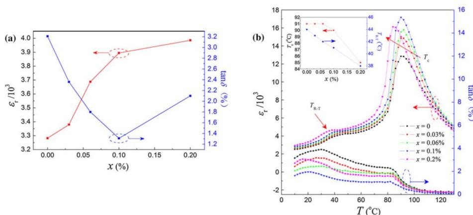
**Figure 10.** (a) Dielectric properties as a function of  $x$  at 1 kHz and (b) temperature dependence of the  $\epsilon_r$  and  $\tan\delta$  of BCZT-xSb ceramics. Reprinted with permission from [78]. Copyright 2011 Springer Nature.
