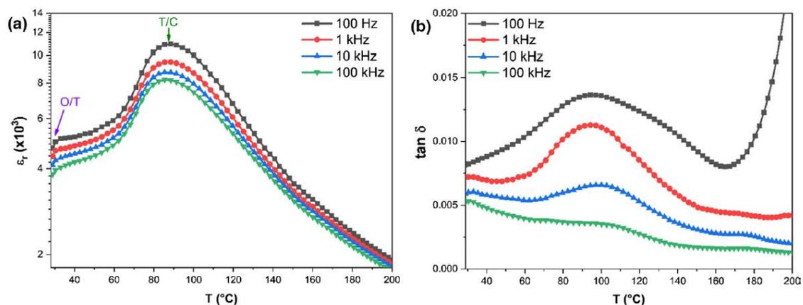
**Figure 4.** Temperature-dependence of the (a) dielectric constant and (b) dielectric loss of  $Ba_{(1-x)}Ca_xZr_yTi_{(1-y)}O_3$  (BCZT) ceramic at different frequencies. O/T corresponds to orthorhombic–tetragonal transition and T/C denotes the tetragonal–cubic phase transition. Reprinted with permission from [55]. Copyright 2019 Springer Nature.
