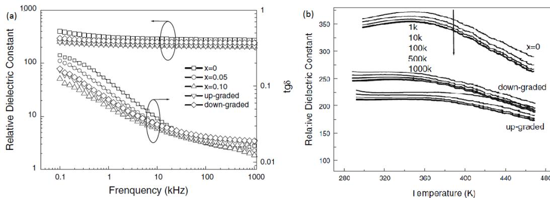
**Figure 11.** The dielectric constant and dielectric loss of the homogenous and compositionally graded BCZT thin films as functions of frequency, measured at room temperature (a). The dielectric constant of  $\text{Ba}_{1-x}\text{Ca}_x\text{Zr}_{0.05}\text{Ti}_{0.95}\text{O}_3$  ( $x = 0$ ) and compositionally graded BCZT thin films as a function of temperature (b). Reprinted with permission from [87]. Copyright 2008 Springer Nature.
