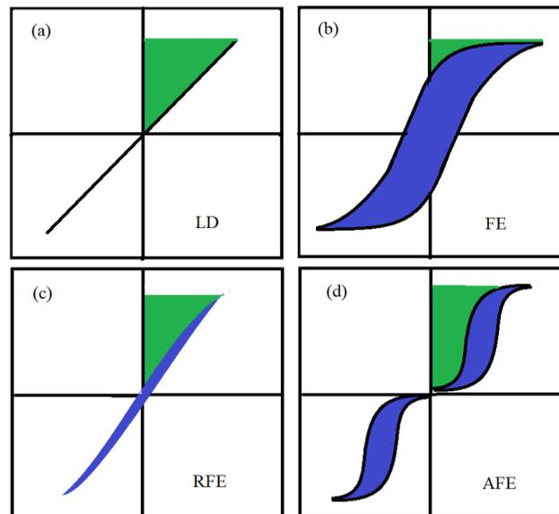
**Figure 1.** Hysteresis and corresponding energy storage density for (a) linear dielectrics, (b) ferroelectrics, (c) relaxor ferroelectrics, and (d) antiferroelectrics. The green area represents energy density and the blue area refers to the energy loss.
