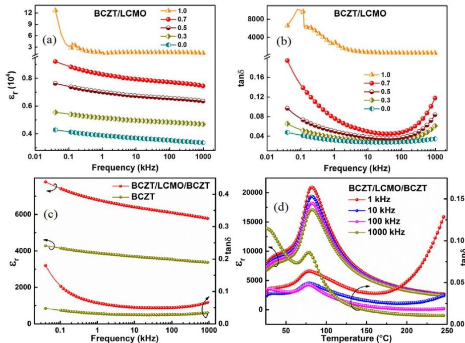
**Figure 19.** Room temperature frequency dependence of  $\epsilon_r$  (a) and  $\tan\delta$  (b) for the  $(1-x)\text{BCZT}-x\text{LCMO}$  laminated composites and frequency (c) and temperature dependence (d) of  $\epsilon_r$  and  $\tan\delta$  for BCZT-LCMO-BCZT composite. Reprinted with permission from [121,122]. Copyright 2017 Elsevier and 2019 AIP Publishing.
