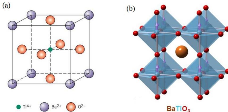
**Figure 2.** The cubic phase for BaTiO<sub>3</sub> unit cell (a). Here Ba<sup>2+</sup> ions occupied the corner of the cube, O<sup>2-</sup> lies in the center of the phases for the composition, Ti<sup>4+</sup> lies in the center of the composition. 3D view of BaTiO<sub>3</sub> perovskite crystal structure (b), image taken from <http://slideplayer.com/slide/9010945/>.
