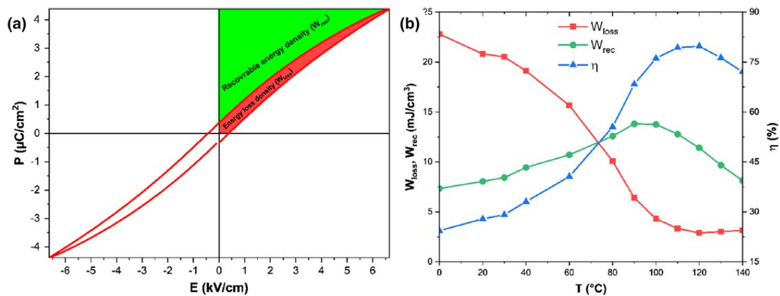
**Figure 5.** P–E loop at 120  $^{\circ}\text{C}$  with schematic calculations energy storage efficiency (a) and variation of recoverable energy density, energy loss density, and the energy storage efficiency of the BCZT ceramic with temperature (b). Reprinted with permission from [55]. Copyright 2019 Springer Nature.
