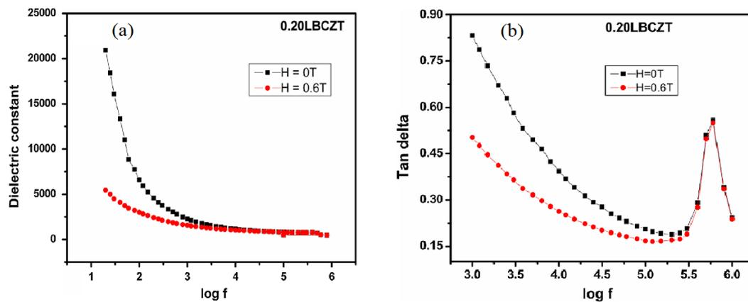
**Figure 7.** (a) Variation of  $\epsilon$  as a function of  $\log f$  for 0.20LBCZT Heterostructure. (b) Variation of  $\tan\delta$  as a function of  $\log f$  for 0.20LBCZT with and without applied magnetic field (H). Reprinted with permission from [51]. Copyright 2016 Springer Nature.
