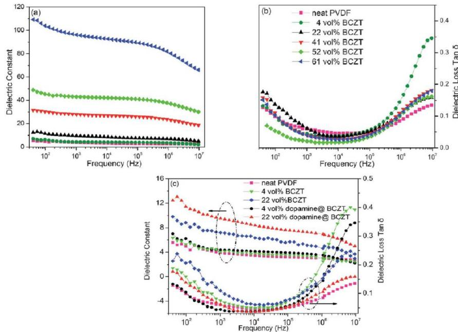
**Figure 14.** Frequency dependence of the dielectric constant (a) and the dielectric loss tangent, (b) of dopamine@BCZT/PVDF composite films, and (c) BCZT/PVDF (Poly(vinylidene fluoride) composite films. Reprinted with permission from [54]. Copyright 2012 Royal Society of Chemistry.
