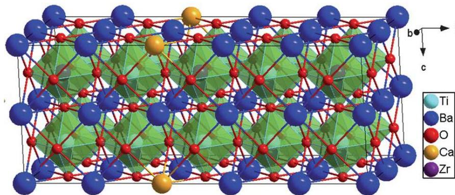
**Figure 3.** Cubic perovskite structure and arrangements of atoms in a  $B_{0.95}C_{0.05}Zr_{0.15}Ti_{0.85}O_3$  supercell with  $5 \times 2 \times 2$  dimension. Reprinted with permission from [54]. Copyright 2012 Royal Society of Chemistry.
