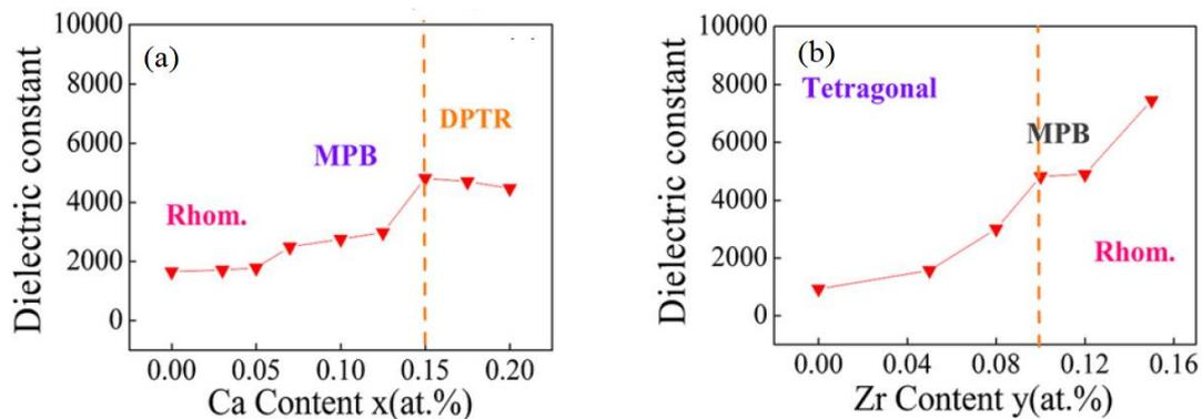
**Figure 6.** (a) The dielectric constant ( $\epsilon_r$ ) of  $(\text{Ba}_{1-x}\text{Ca}_x)(\text{Zr}_{0.1}\text{Ti}_{0.9})\text{O}_3$  ceramics. (b) The dielectric constant ( $\epsilon_r$ ) of  $(\text{Ba}_{0.85}\text{Ca}_{0.15})(\text{Zr}_y\text{Ti}_{1-y})\text{O}_3$  ceramics. For different acronyms in the figures, please see the text. Reprinted with permission from [57]. Copyright 2012 The American Ceramic Society.
