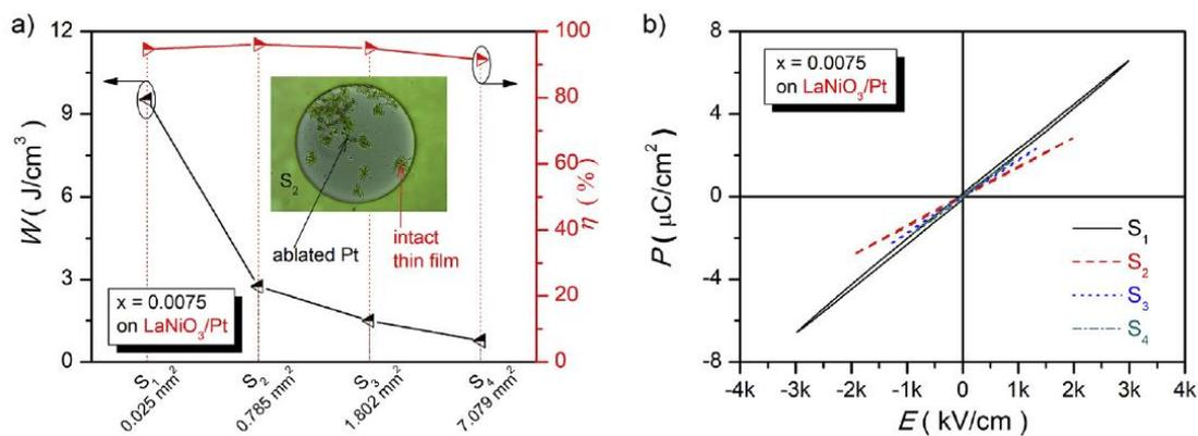
**Figure 17.** La-doped BCZT thin films at  $x = 0.0075$  on  $\text{LaNiO}_3/\text{Pt}$  composite bottom electrodes. The area of top electrode as a function of  $W$  and  $\eta$ . Inset: image of Pt top electrode (a). Polarization-electric field ( $P$ - $E$ ) loops with various sizes of Pt top electrodes (b). Reprinted with permission from [62]. Copyright 2019 Elsevier.
