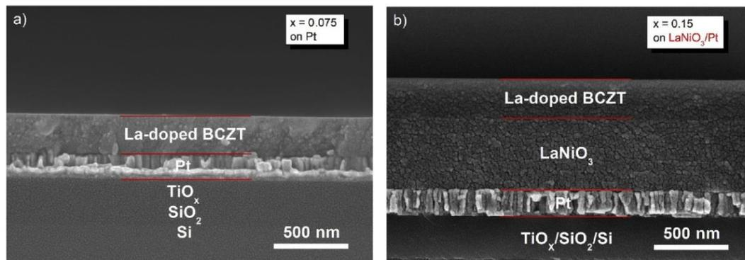
**Figure 16.** Cross-sectional SEM images of La-doped BCZT thin films at  $x = 0.0075$  and  $0.15$ . (a) On Pt bottom electrodes, and (b) on  $\text{LaNiO}_3/\text{Pt}$  composite bottom electrodes. Reprinted with permission from [62]. Copyright 2019 Elsevier.
