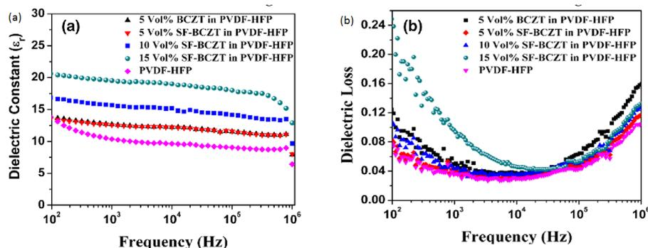
**Figure 15.** Dielectric constant versus frequency (a), dielectric loss versus frequency (b) for different molar concentration of PVDF-HFP in BCZT. Reprinted with permission from [61]. Copyright 2018 Springer Nature.
