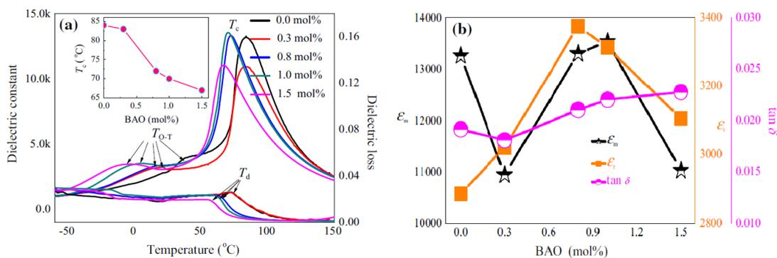
**Figure 8.** The temperature dependence of  $\epsilon_r$  and  $T_C$  for  $(1-x)\text{BCZT}-x\text{BAO}$  ceramics measured at 1 kHz (a). The maximum dielectric constant ( $\epsilon_m$ ), dielectric constant ( $\epsilon_r$ ), and dielectric loss ( $\tan\delta$ ) of BCZT ceramics with different BAO contents (b). Reprinted with permission from [76]. Copyright 2015 Springer Nature.
