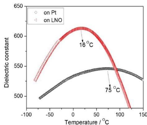
**Figure 12.** Dielectric constant as a function of temperature measured at frequency of 100 kHz for the BCZT thin films deposited on Pt(111)/Ti/SiO<sub>2</sub>/Si substrate and LNO/Pt(111)/Ti/SiO<sub>2</sub>/Si substrate. Reprinted with permission from [60]. Copyright 2013 Elsevier.
