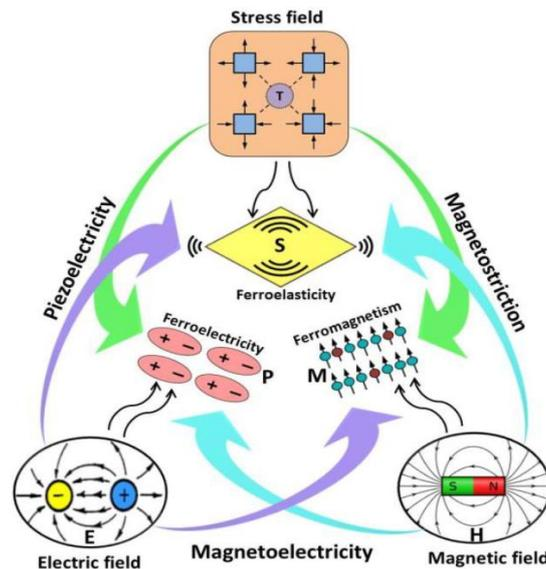
**Figure 18.** Schematic illustration of magnetic-elastic-electric couplings in multiferroic materials. Here, M is magnetization, S is mechanical strain, and P is dielectric polarization. Reprinted with permission from [103]. Copyright 2019 MDPI Publishers.
