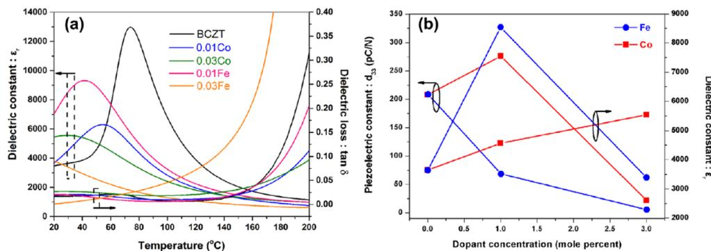
**Figure 9.** Dielectric and piezoelectric properties of BCZT-xCo and BCZT-xFe ceramics. Dielectric versus temperature at 1 kHz (a) and piezoelectric constant as a function of dopant concentration (b). Reprinted with permission from [71]. Copyright 2018 WILEY-VCH Verlag GmbH & Co.
