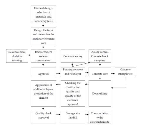
Figure 1. Process of manufacturing of prefabricated wall elements [30].
