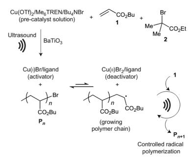
**Figure 2.** Mechanism of ultrasound-induced ATRP of BA 1 starting from the alkyl halide initiator 2 with the use of  $BaTiO_3$  piezoelectric nanoparticles [48]. Reprinted with permission from Springer Nature. Copyright 2016.
