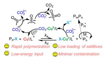
**Figure 7.** Mechanism of ultrasonication-induced ATRP with catalytic activation-mediated by carbonates [52]. Reprinted with permission from American Chemical Society. Copyright 2019.
