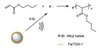
**Figure 5.** Mechanically controlled free-radical polymerization of BA [50]. Reprinted with permission from Wiley-VCH Verlag GmbH and Co. KGaA, Weinheim. Copyright 2019.
