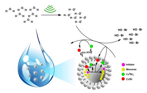
**Figure 8.** Ultrasound-mediated ATRP in a miniemulsion by interfacial and ion-pair catalysis [12]. Reprinted with permission from WILEY-VCH Verlag GmbH and Co. KGaA, Weinheim. Copyright 2019.
