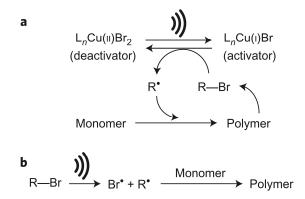
**Figure 1.** Two potential routes for the initiation of polymerization process by ultrasound agitation: (**a**) reduction of deactivator by the piezocatalytic effect resulting in the formation of an activator followed by radical generation, and thus growing of the polymer chain; (**b**) sonication-mediated generation of radicals, directly initiating a radical polymerization [48]. Reprinted with permission from Springer Nature. Copyright 2016.
