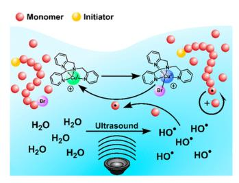
**Figure 6.** Mechanism of ultrasonication-induced ATRP [43]. Reprinted with permission from American Chemical Society. Copyright 2018.
