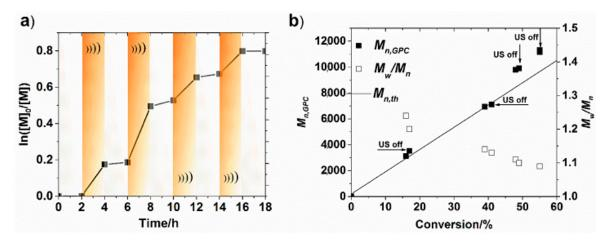
**Figure 3.** Temporally controlled mechano-ATRP approach in the polymerization of methyl acrylate (MA): (a) first-order kinetics plot, (b) evolution of molecular weight and dispersity of prepared polymers [41]. Reprinted with permission from American Chemical Society. Copyright 2017.
