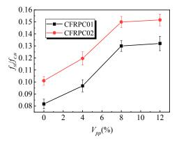
Figure 11. Effect of the polymer-cement ratio on the tension-compression ratio of specimens.
