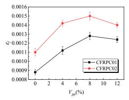
Figure 7. Effect of the polymer-cement ratio on the peak strain in the flexural test.
