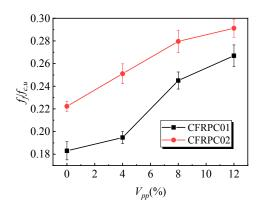
Figure 8. Effect of the polymer-cement ratio on the flexural-compressive ratio of the specimens.
