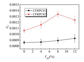
**Figure 10.** Effect of the polymer–cement ratio on the peak strain of the specimens in the splitting tensile test.
