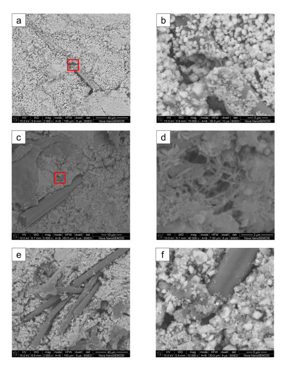
Figure 12. Polymers with different morphologies in the fiber transition zone. (a) Granular polymer; (b) a  $5 \times$  enlargement of (a); (c) fibrous polymer; (d) an  $8 \times$  times enlargement of (b); (e) membranous polymer on exposed fibers; (f) membranous polymer at the fiber–matrix interface.
