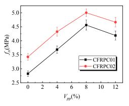
Figure 9. Effect of the polymer–cement ratio on the splitting tensile strength.
