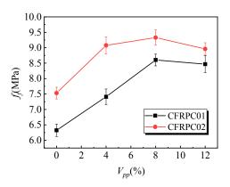
Figure 6. Effect of the polymer-cement ratio on the flexural strength of the specimens.
