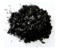
Figure 3. Short-cut carbon fibers.
