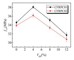
Figure 4. Effect of the polymer-cement ratio on the compressive strength of the specimens.
