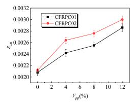
Figure 5. Effect of the polymer-cement ratio on the peak compressive strain of the specimens.
