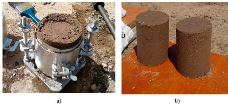
Figure 6. Preparation of the samples made of fine aggregate with cement: cylindric form (a); samples (b).
