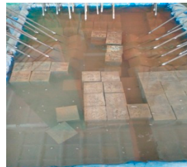
Figure 3. Specimens cured under water in tank.
