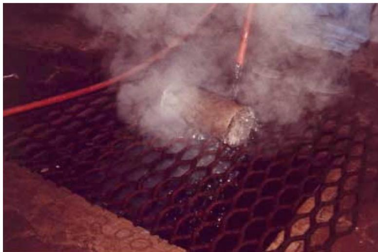
**Figure 2.** Subtle cooling of test specimens by water aspersion.
