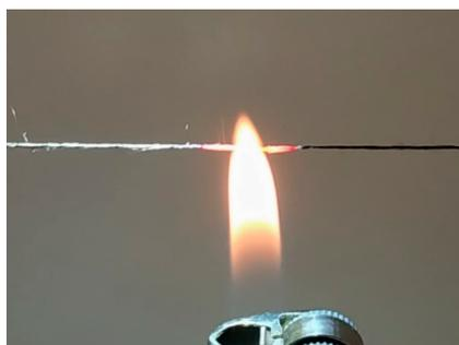
**Figure 11.** “Lola-M” fiber behavior in open flame.
