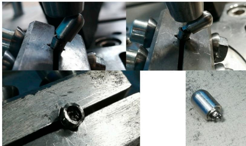
**Figure 17.** Failure of third implant during fatigue testing.
