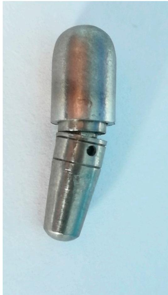
**Figure 16.** Failure of second tested implant due to test machine-related problems.
