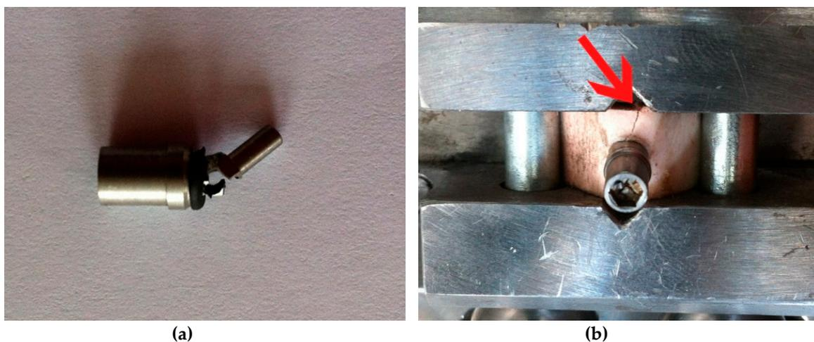
**Figure 10.** (a) Abutment fracture in P2 implant; (b) fissure of the bone around P1 implant.
