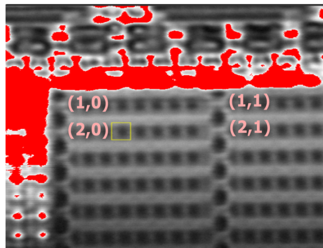
Figure 4. Schematic of SRAM words in a SRAM block.
