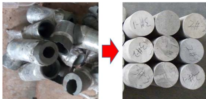
Figure 3. The coal gangue specimens for compressive test.
