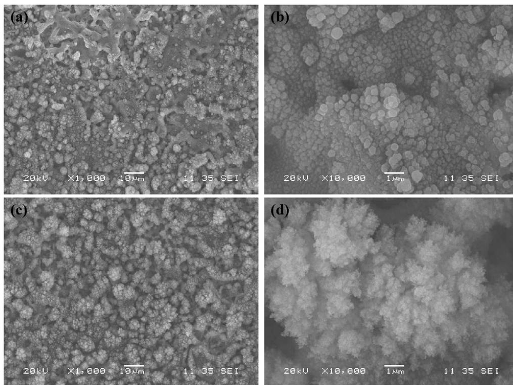
**Figure 6.** Surface structure of the coatings deposited without a quartz tube surrounding the jet (a,b) and with the quartz tube (c,d).
