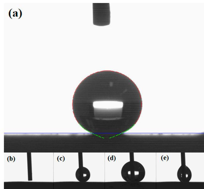
**Figure 14.** (a) a demonstration of the Tangent approximation method and (b–e) the procedure for determination of advancing and receding angles.
