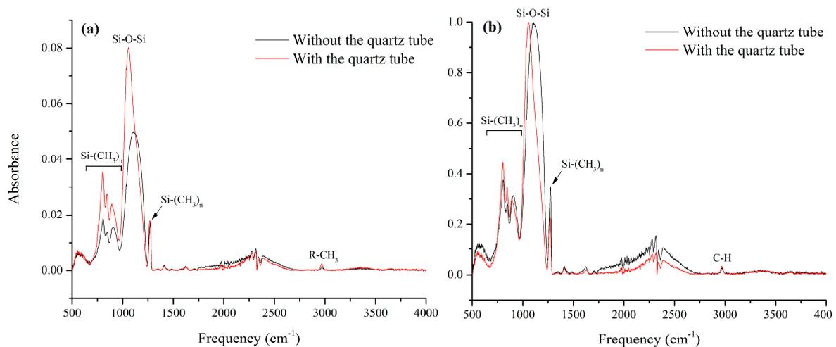
**Figure 5.** (a) Fourier transform infrared spectroscopy (FTIR) spectra of samples prepared with PT5 conditions, with and without the quartz tube surrounding the jet. (b) shows the same spectra normalized according to Si-O-Si band.
