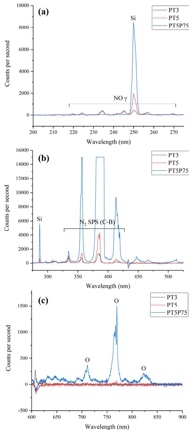
**Figure 7.** Optical emission spectra from PT3, PT5, and PT5P75 conditions. Three ranges of wavelength are chosen to highlight some of the differences. (a) 200–275 nm, (b) 275–525 nm, and (c) 600–900 nm.
