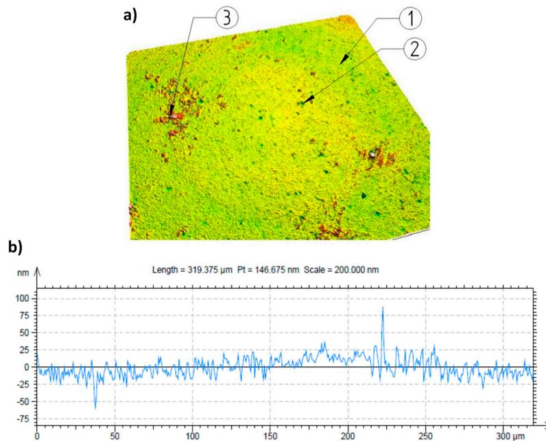
**Figure 4.** Surface structure of the burnishing ball made from  $\text{Si}_3\text{N}_4$ : (a) Surface photograph; (b) surface profile, 1—surface structure, 2—small pores occurring on the surface, 3—additional material on the ball surface.
