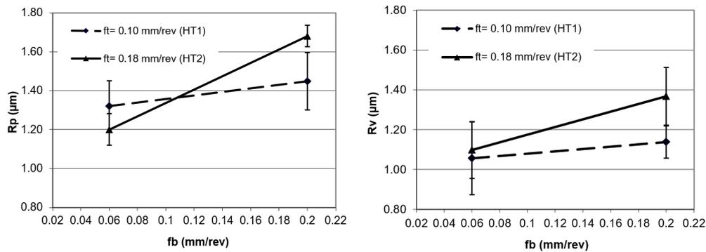
**Figure 7.** Surface roughness after burnishing; Rp and Rv are parameters as a function of feed rate.
