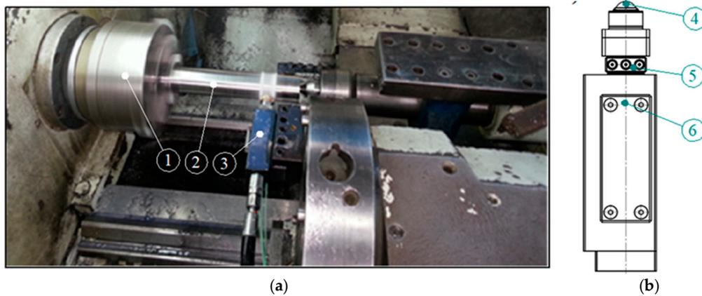
**Figure 3.** Burnishing a shaft on a computerized numerical control (CNC) lathe: (a) View of the burnishing process; (b) schematic drawing of a hydrostatic burnishing tool with a “Kistler” sensor, 1—a spindle with a chuck, 2—the workpiece, 3—a burnishing tool, 4—the burnishing ball, 5—a force sensor, 6—a shank with hydraulic pressure.
