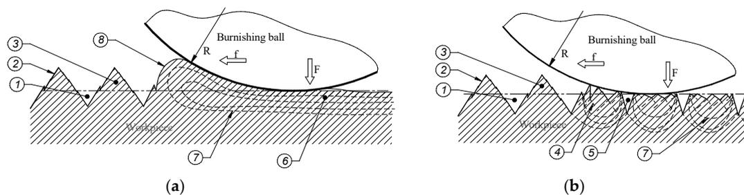
**Figure 1.** Schematic drawing of a burnishing process: (a) Soft materials; (b) hard materials, 1—valley of roughness, 2—surface profile, 3—peak of roughness, 4—slip plane, 5—deep valley after burnishing, 6—zone of material deformation, 7—zone of plastic and elastic deformation, 8—wave of material in front of the burnishing tool.
