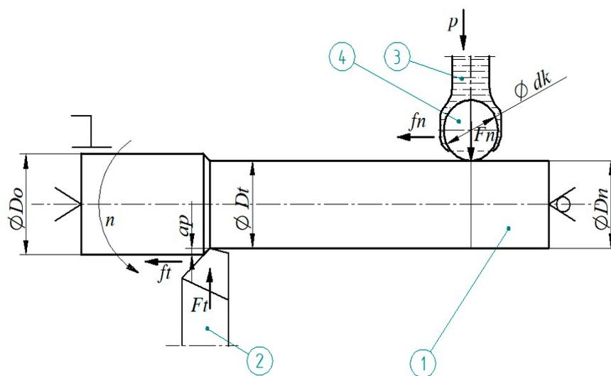
**Figure 2.** Schematic drawing of a machining process: 1—machined shaft, 2—tool for hard turning, 3—processing liquid, 4—burnishing ball,  $f_t$ —turning feed,  $a_p$ —depth of turning,  $D_o$ —diameter of the processed shaft,  $D_t$ —shaft diameter after turning,  $D_n$ —shaft diameter after burnishing,  $F_n$ —burnishing force,  $f_n$ —burnishing feed,  $p$ —pressure of the processing liquid,  $d_k$ —diameter of the burnishing ball.
