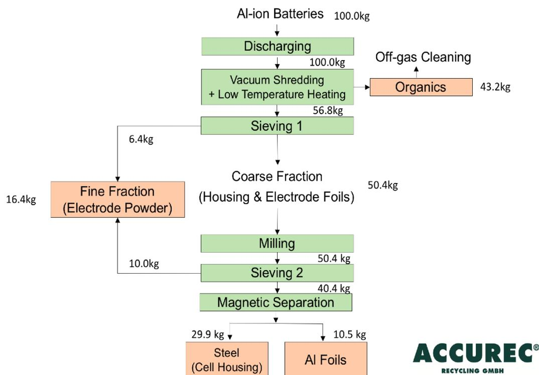
**Figure S3.** Recycling steps designed by ACCUREC for the Li-ion cell [9].
