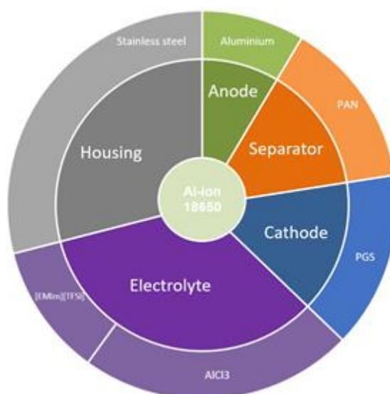
Figure S1. 18650 Al-ion cell composition by components and materials.
