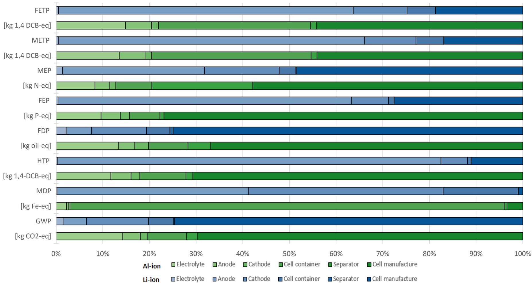
**Figure S7.** Production phase contribution analysis for eight impact categories of Li-ion and Al-ion 18650 cells.
