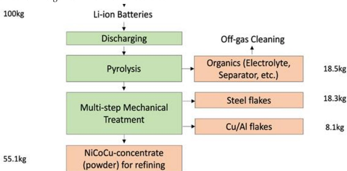
Figure S6. Recycling steps designed by ACCUREC for the Li-ion cell [9].
