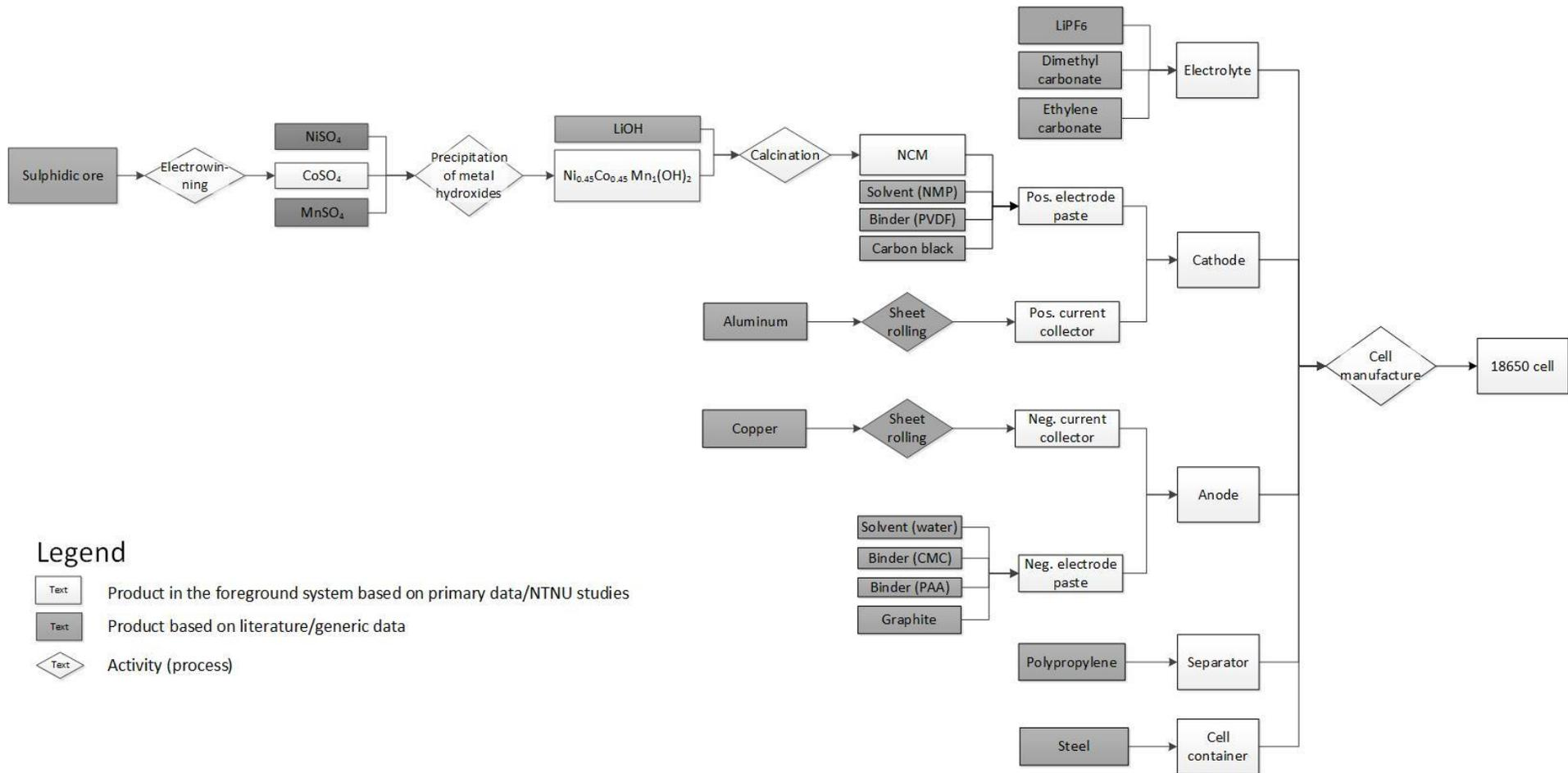
Figure S5. Flowchart for the production of the 18650 Li-ion battery cell.
