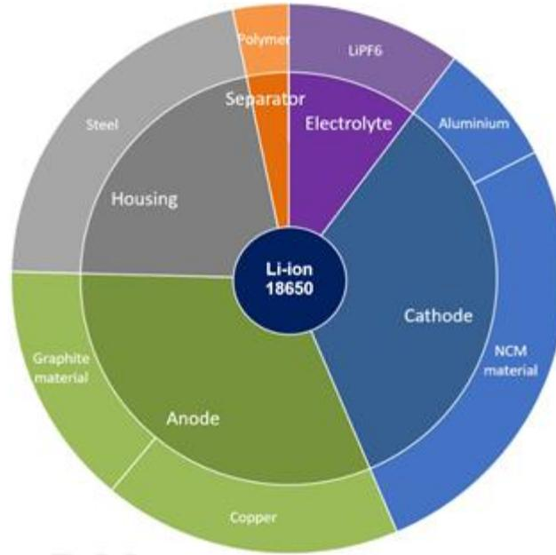
**Figure S4.** 18650 Li-ion cell composition by components and materials.
